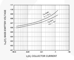
Figure 3. Base-Emitter Voltage
