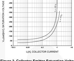
Figure 2. Collector-Emitter Saturation Voltage
