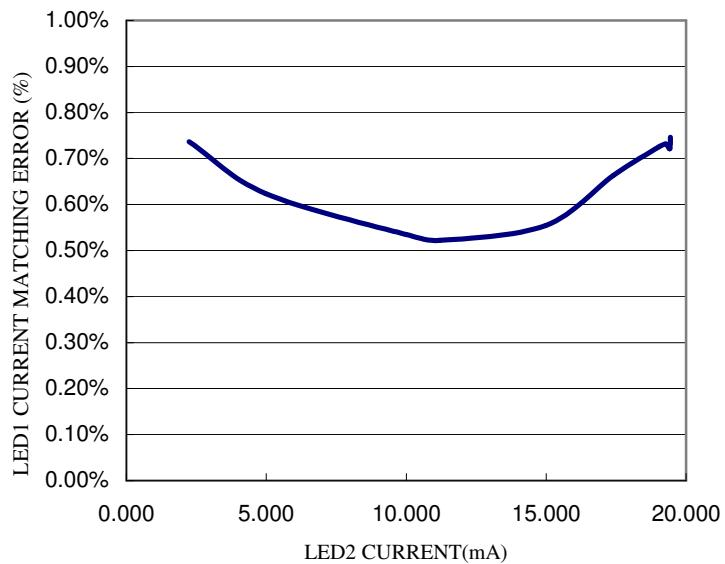
Figure 3. Typical current matching between LED1 and LED2
