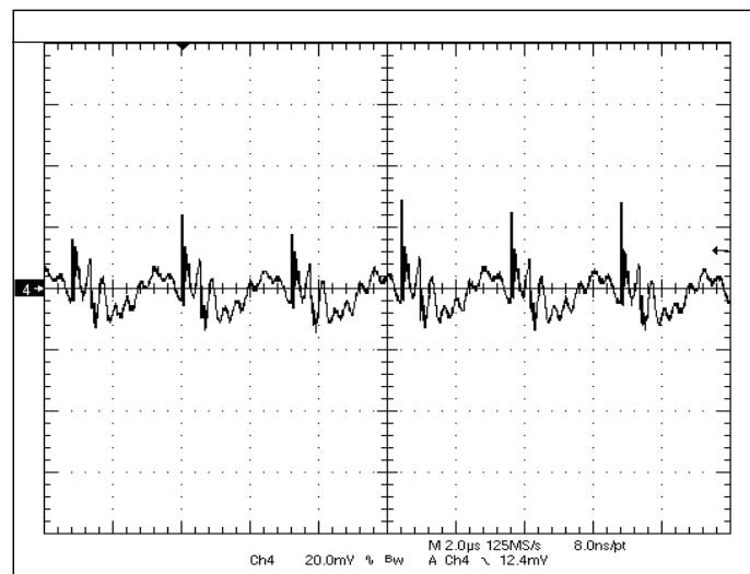
**Fig 1.8V-5:** Output voltage ripple (20mV/div.) for  $V_{out}=1.8V$  at full rated load current into a resistive load with external capacitance  $47\mu Fx2$  ceramic +  $1\mu F$  ceramic at  $V_{in}=12V$ .
