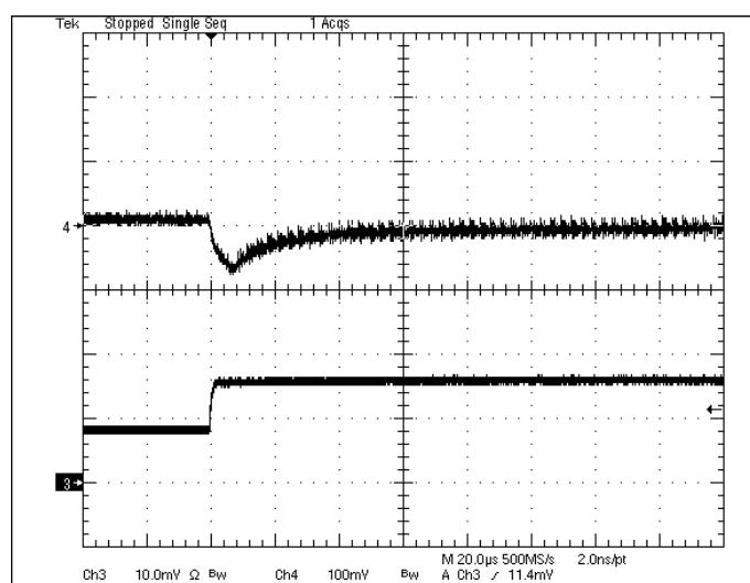
**Fig 1.5V-6:** Output voltage response for  $V_{out}=1.5V$  to positive load current step change from 4A to 8A with slew rate of  $5A/\mu s$  at  $V_{in}=12V$ .  $C_o=47\mu Fx2$  ceramic.
