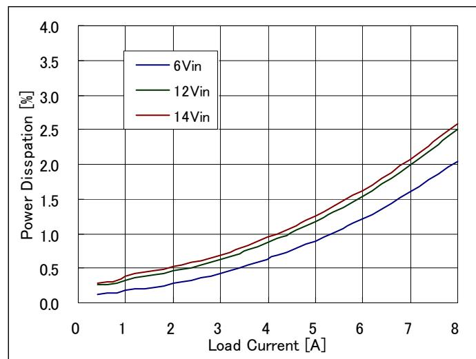
**Fig 1.2V-3:** Power Loss vs. load current and input voltage for  $V_{out}=1.2V$ .
