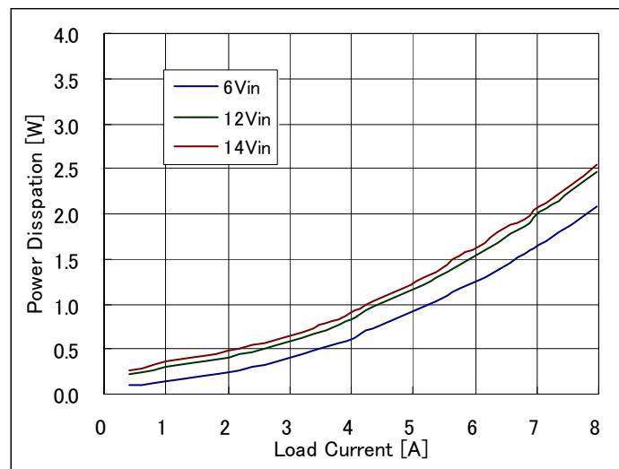
**Fig 1.0V-3:** Power Loss vs. load current and input voltage for  $V_{out}=1.0V$ .
