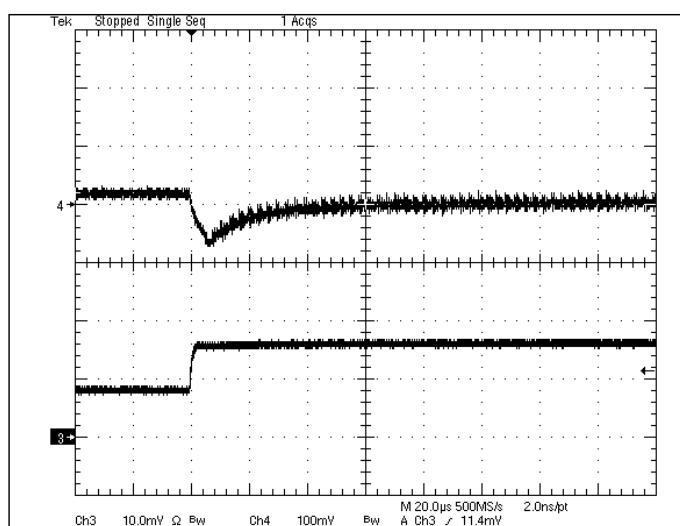
**Fig 1.2V-6:** Output voltage response for  $V_{out}=1.2V$  to positive load current step change from 4A to 8A with slew rate of  $5A/\mu s$  at  $V_{in}=12V$ .  $C_o=47\mu Fx2$  ceramic.
