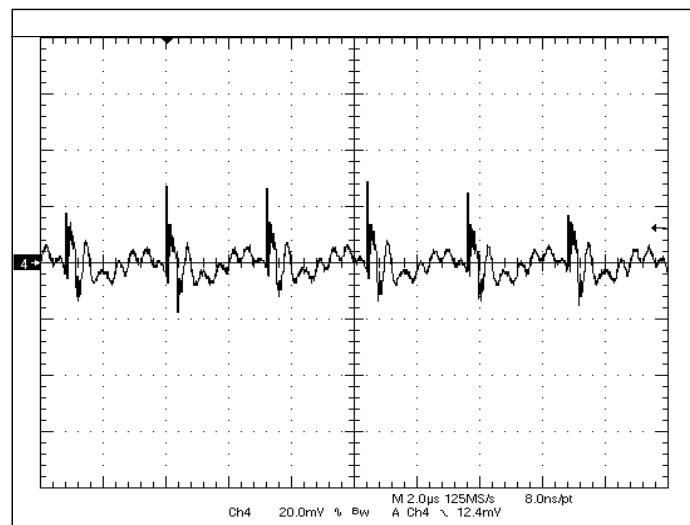
**Fig 1.0V-5:** Output voltage ripple (20mV/div.) for  $V_{out}=1.0V$  at full rated load current into a resistive load with external capacitance  $47\mu Fx2$  ceramic +  $1\mu F$  ceramic at  $V_{in}=12V$ .
