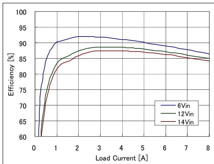
**Fig 1.8V-2:** Efficiency vs. load current and input voltage for  $V_{out}=1.8V$ .
