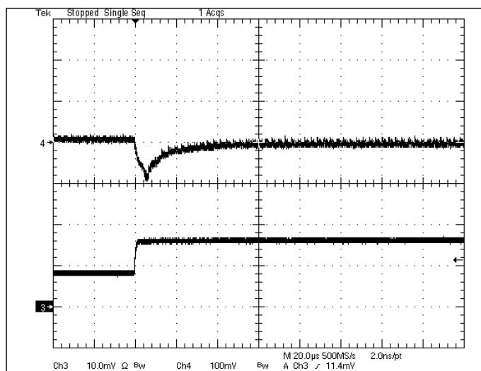
**Fig 2.5V-6:** Output voltage response for  $V_{out}=2.5V$  to positive load current step change from 4A to 8A with slew rate of  $5A/\mu s$  at  $V_{in}=12V$ .  $C_o=47\mu Fx2$  ceramic.
