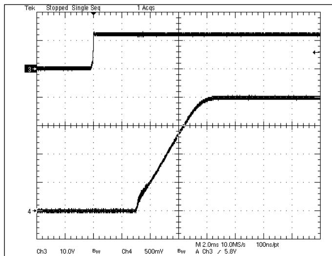
**Fig 2.0V-4:** Turn-on transient for  $V_{out}=2.0V$  with application of  $V_{in}$  at full rated load current (resistive) and  $47\mu Fx2$  external capacitance at  $V_{in}=12V$ .
