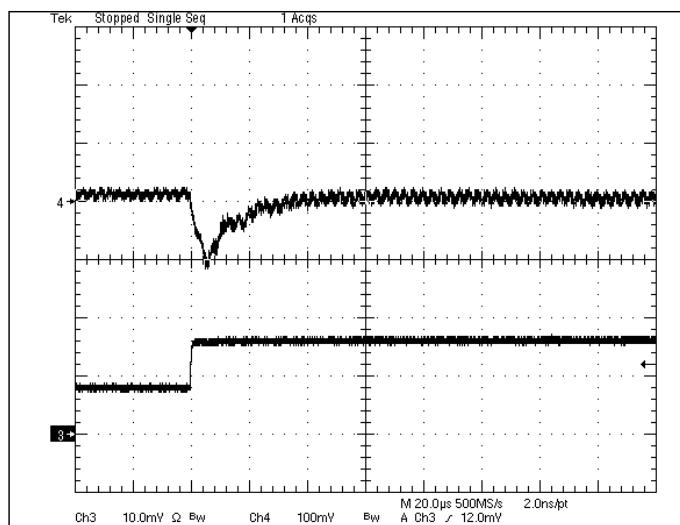
**Fig 5.0V-6:** Output voltage response for  $V_{out}=5.0V$  to positive load current step change from 4A to 8A with slew rate of  $5A/\mu s$  at  $V_{in}=12V$ .  $C_o=47\mu Fx2$  ceramic.
