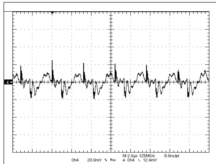
**Fig 3.3V-5:** Output voltage ripple (20mV/div.) for  $V_{out}=3.3V$  at full rated load current into a resistive load with external capacitance  $47\mu Fx2$  ceramic +  $1\mu F$  ceramic at  $V_{in}=12V$ .
