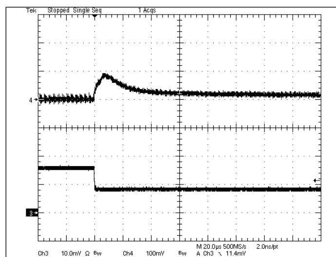
**Fig 1.0V-7:** Output voltage response for  $V_{out}=1.0V$  to negative load current step change from 8A to 4A with slew rate of  $-5A/\mu s$  at  $V_{in}=12V$ .  $C_o=47\mu Fx2$  ceramic.
