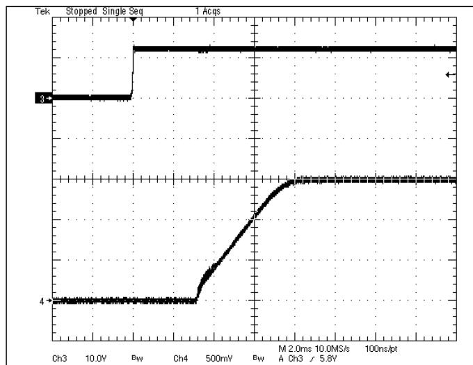
**Fig 1.5V-4:** Turn-on transient for  $V_{out}=1.5V$  with application of  $V_{in}$  at full rated load current (resistive) and  $47\mu Fx2$  external capacitance at  $V_{in}=12V$ .
