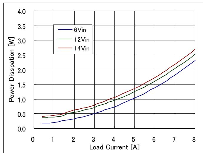
**Fig 2.0V-3:** Power Loss vs. load current and input voltage for  $V_{out}=2.0V$ .
