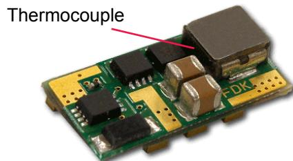
Fig. C: Location of the thermocouple for thermal testing
