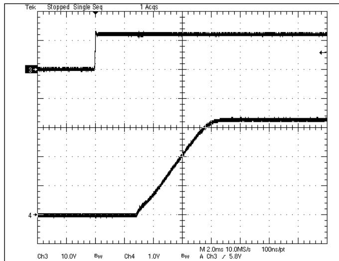
**Fig 3.3V-4:** Turn-on transient for  $V_{out}=3.3V$  with application of  $V_{in}$  at full rated load current (resistive) and  $47\mu Fx2$  external capacitance at  $V_{in}=12V$ .
