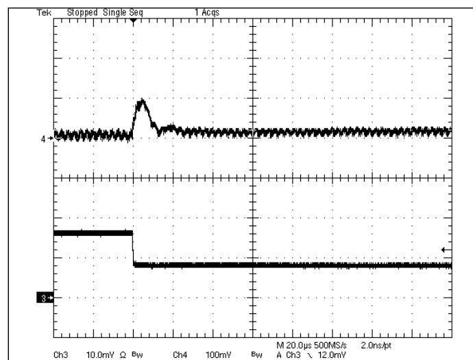
**Fig 5.0V-7:** Output voltage response for  $V_{out}=5.0V$  to negative load current step change from 8A to 4A with slew rate of  $-5A/\mu s$  at  $V_{in}=12V$ .  $C_o=47\mu Fx2$  ceramic.
