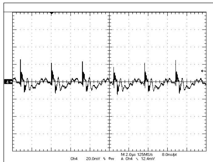
**Fig 1.2V-5:** Output voltage ripple (20mV/div.) for  $V_{out}=1.2V$  at full rated load current into a resistive load with external capacitance  $47\mu Fx2$  ceramic +  $1\mu F$  ceramic at  $V_{in}=12V$ .
