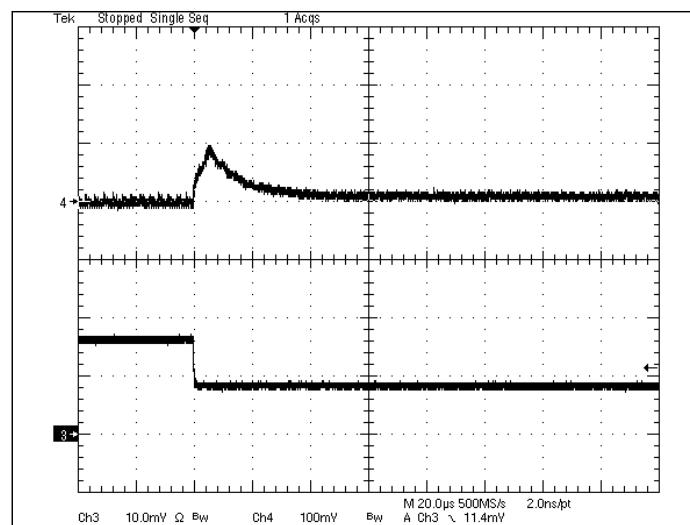
**Fig 2.5V-7:** Output voltage response for  $V_{out}=2.5V$  to negative load current step change from 8A to 4A with slew rate of  $-5A/\mu s$  at  $V_{in}=12V$ .  $C_o=47\mu Fx2$  ceramic.
