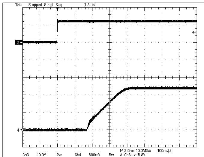
**Fig 1.2V-4:** Turn-on transient for  $V_{out}=1.2V$  with application of  $V_{in}$  at full rated load current (resistive) and  $47\mu Fx2$  external capacitance at  $V_{in}=12V$ .
