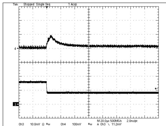
**Fig 2.0V-7:** Output voltage response for  $V_{out}=2.0V$  to negative load current step change from 8A to 4A with slew rate of  $-5A/\mu s$  at  $V_{in}=12V$ .  $C_o=47\mu Fx2$  ceramic.
