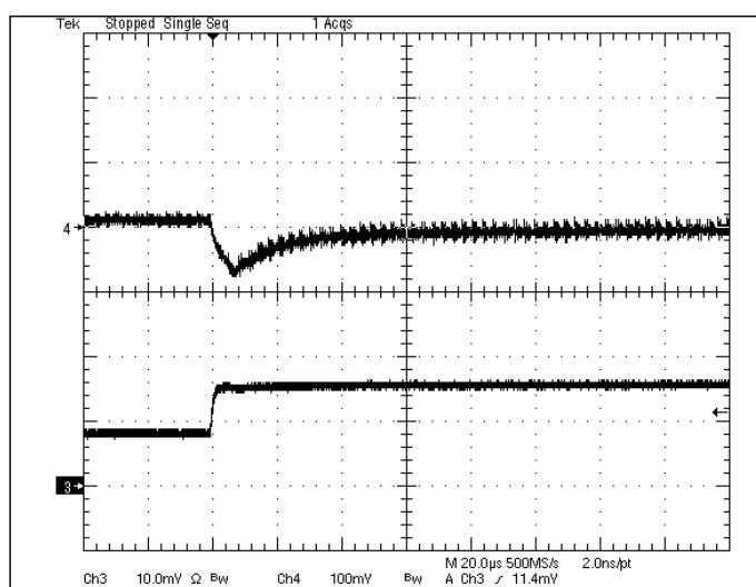
**Fig 1.0V-6:** Output voltage response for  $V_{out}=1.0V$  to positive load current step change from 4A to 8A with slew rate of  $5A/\mu s$  at  $V_{in}=12V$ .  $C_o=47\mu Fx2$  ceramic.
