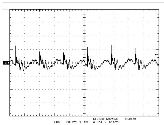
**Fig 1.5V-5:** Output voltage ripple (20mV/div.) for  $V_{out}=1.5V$  at full rated load current into a resistive load with external capacitance  $47\mu Fx2$  ceramic +  $1\mu F$  ceramic at  $V_{in}=12V$ .
