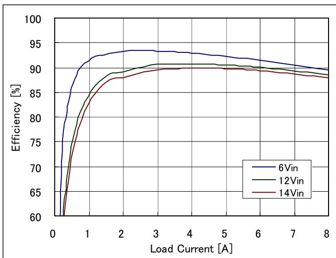
**Fig 2.5V-2:** Efficiency vs. load current and input voltage for  $V_{out}=2.5V$ .
