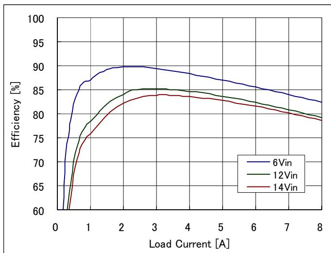
**Fig 1.2V-2:** Efficiency vs. load current and input voltage for  $V_{out}=1.2V$ .
