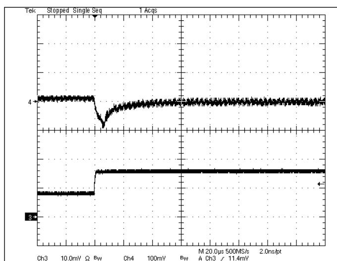
**Fig 3.3V-6:** Output voltage response for  $V_{out}=3.3V$  to positive load current step change from 4A to 8A with slew rate of  $5A/\mu s$  at  $V_{in}=12V$ .  $C_o=47\mu Fx2$  ceramic.
