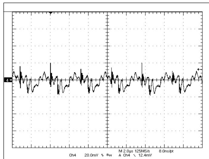
**Fig 2.5V-5:** Output voltage ripple (20mV/div.) for  $V_{out}=2.5V$  at full rated load current into a resistive load with external capacitance  $47\mu Fx2$  ceramic +  $1\mu F$  ceramic at  $V_{in}=12V$ .
