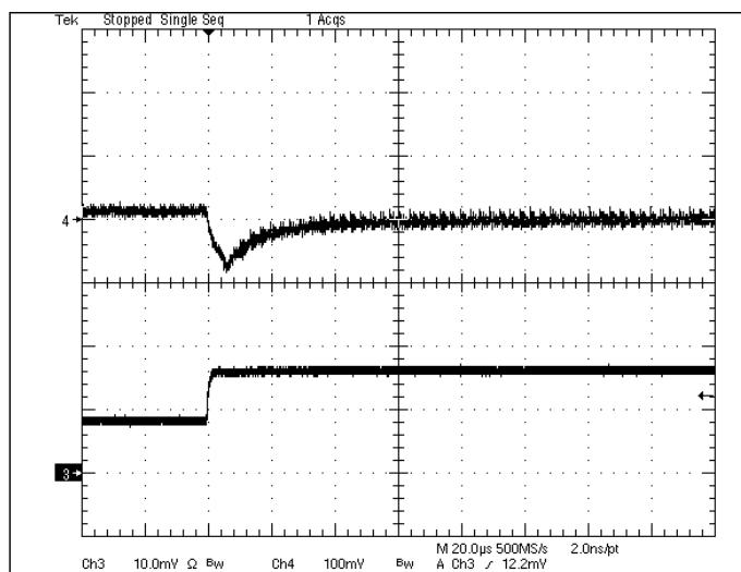
**Fig 1.8V-6:** Output voltage response for  $V_{out}=1.8V$  to positive load current step change from 4A to 8A with slew rate of  $5A/\mu s$  at  $V_{in}=12V$ .  $C_o=47\mu Fx2$  ceramic.
