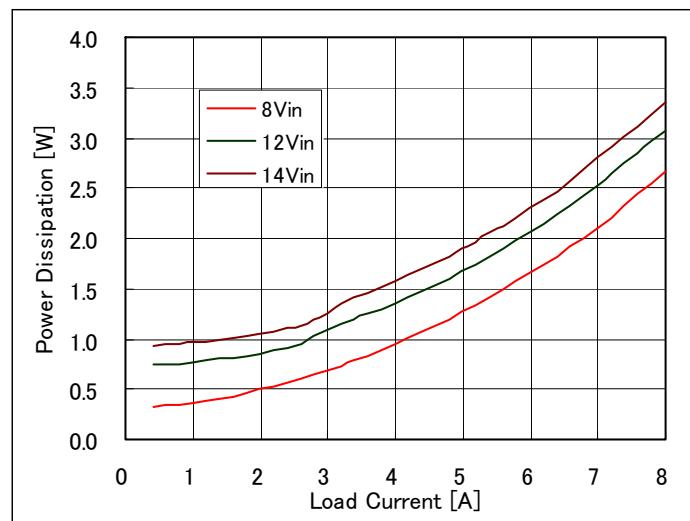
**Fig 5.0V-3:** Power Loss vs. load current and input voltage for  $V_{out}=5.0V$ .
