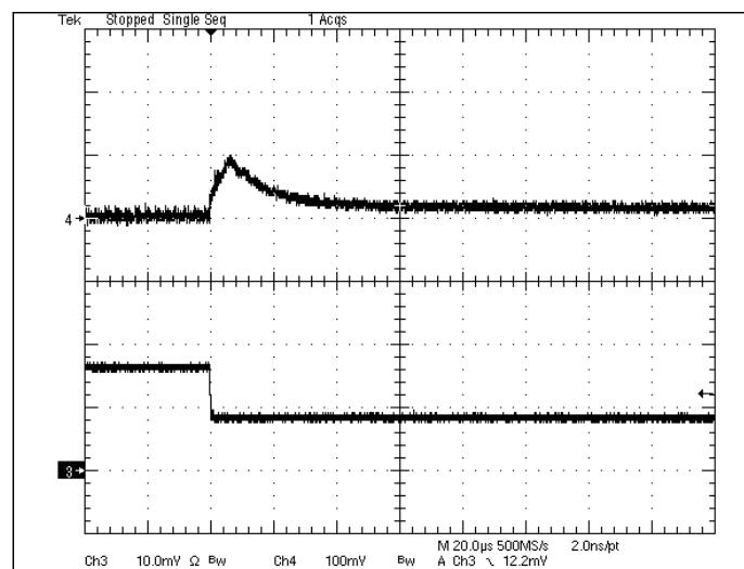
**Fig 1.8V-7:** Output voltage response for  $V_{out}=1.8V$  to negative load current step change from 8A to 4A with slew rate of  $-5A/\mu s$  at  $V_{in}=12V$ .  $C_o=47\mu Fx2$  ceramic.
