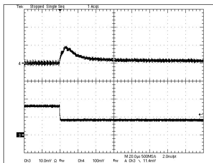
**Fig 1.5V-7:** Output voltage response for  $V_{out}=1.5V$  to negative load current step change from 8A to 4A with slew rate of  $-5A/\mu s$  at  $V_{in}=12V$ .  $C_o=47\mu Fx2$  ceramic.
