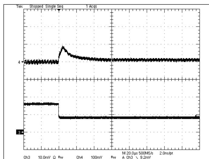
**Fig 3.3V-7:** Output voltage response for  $V_{out}=3.3V$  to negative load current step change from 8A to 4A with slew rate of  $-5A/\mu s$  at  $V_{in}=12V$ .  $C_o=47\mu Fx2$  ceramic.
