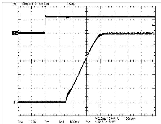
**Fig 2.5V-4:** Turn-on transient for  $V_{out}=2.5V$  with application of  $V_{in}$  at full rated load current (resistive) and  $47\mu Fx2$  external capacitance at  $V_{in}=12V$ .
