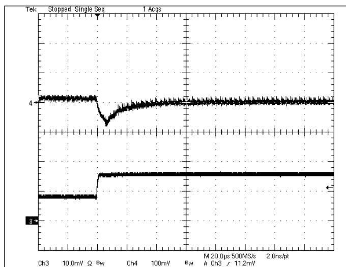
**Fig 2.0V-6:** Output voltage response for  $V_{out}=2.0V$  to positive load current step change from 4A to 8A with slew rate of  $5A/\mu s$  at  $V_{in}=12V$ .  $C_o=47\mu Fx2$  ceramic.
