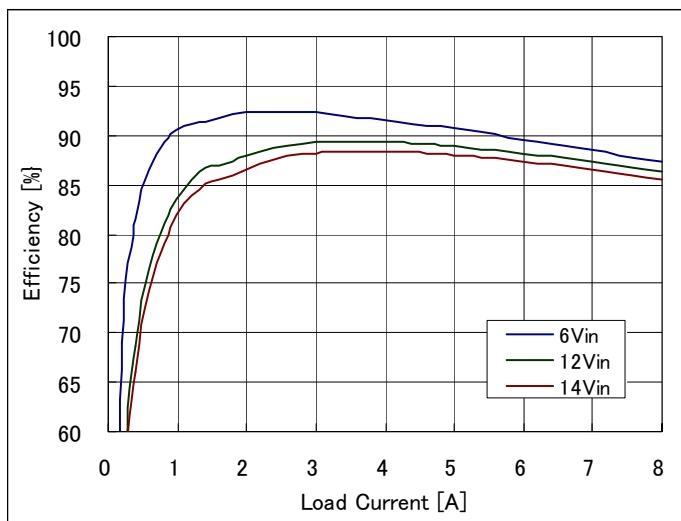
**Fig 2.0V-2:** Efficiency vs. load current and input voltage for  $V_{out}=2.0V$ .
