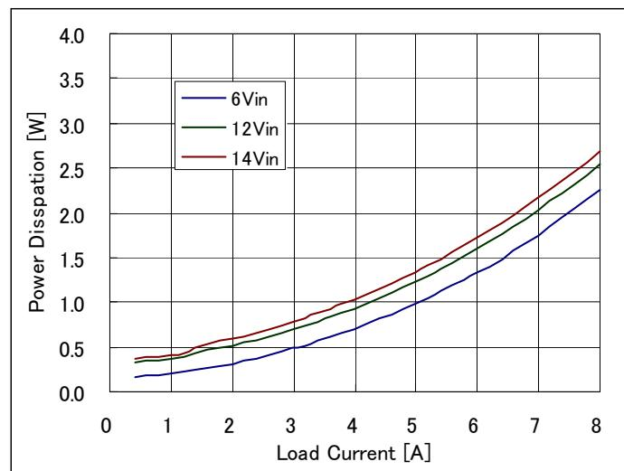
**Fig 1.8V-3:** Power Loss vs. load current and input voltage for  $V_{out}=1.8V$ .
