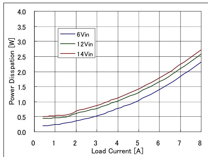
**Fig 2.5V-3:** Power Loss vs. load current and input voltage for  $V_{out}=2.5V$ .
