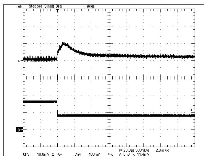
**Fig 1.2V-7:** Output voltage response for  $V_{out}=1.2V$  to negative load current step change from 8A to 4A with slew rate of  $-5A/\mu s$  at  $V_{in}=12V$ .  $C_o=47\mu Fx2$  ceramic.
