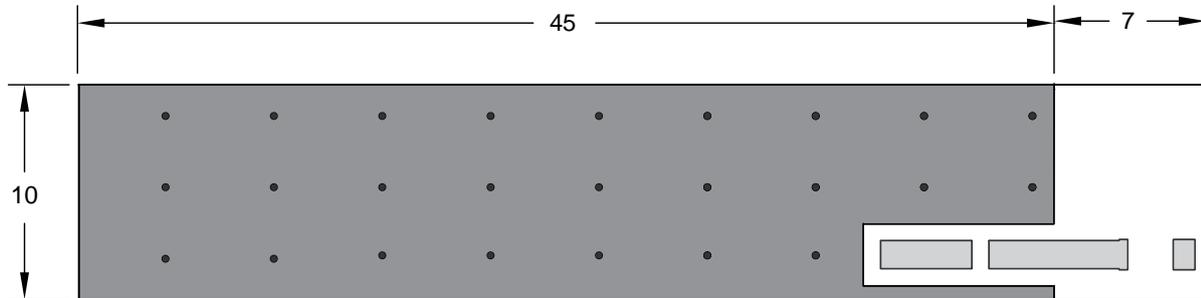
**Fig. 3** Outlook and dimension of evaluation board
