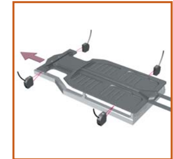
Measuring Car Body Widths (ZS-HLDS10)
