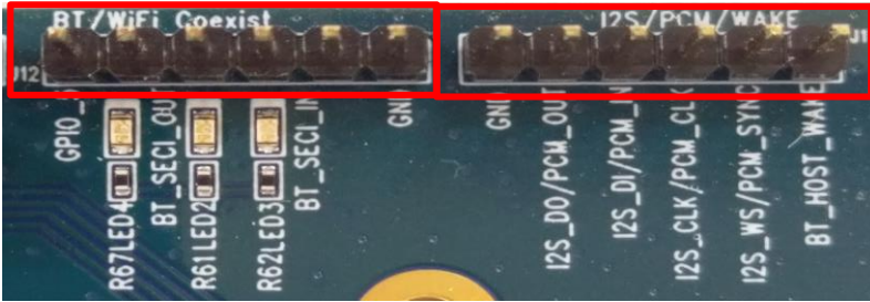
Figure 2: Pin headers - J11 and J12
