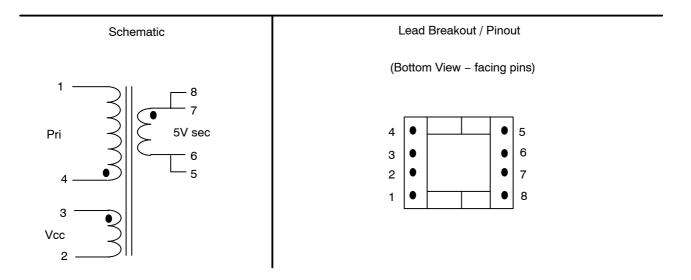
Figure 4. DCM Flyback Transformer Design
