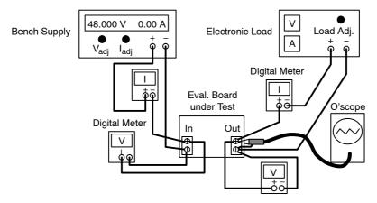
Figure 6. Setup Procedure Diagram
