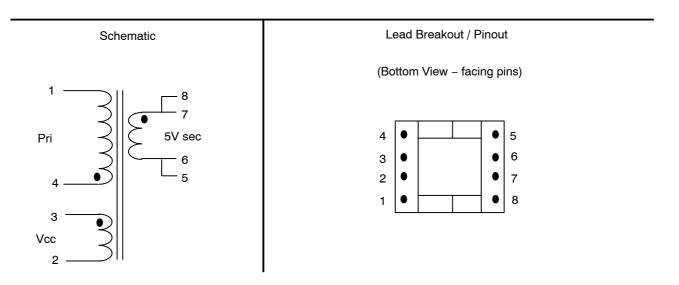
Figure 5. CCM Flyback Transformer Design
