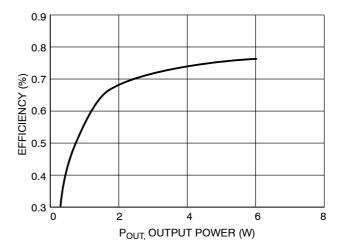
Figure 2. Efficiency Versus Output Power Graph
