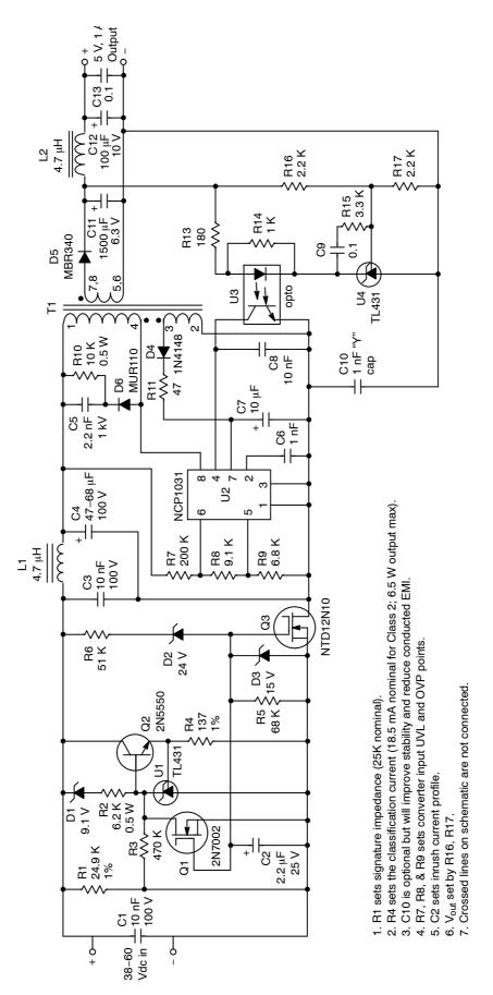
Figure 3. Schematic for the NCP1031 Evaluation Board
