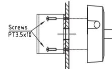
3. Press the shaft (L=52AD11) into the switch. Connect the wires to the terminals.
