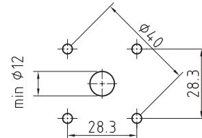
2. Fix the handle LK11 and the OKA door mounting kit to the door.
