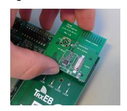
Insert a CC110LEM into the TrxEB. The connectors will only fit in one position so that the EM cannot be inserted the wrong way. Do not use excessive force on the EM.
