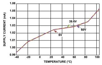
FIGURE 35. V3P3 SUPPLY CURRENT vs TEMPERATURE
