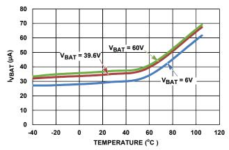
FIGURE 28. PACK VOLTAGE SLEEP CURRENT vs TEMPERATURE AT 6V, 39.6V, 60V (DAISY CHAIN TOP)
