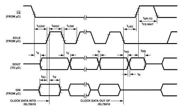
FIGURE 3. SPI FULL DUPLEX (4-WIRE) INTERFACE TIMING
