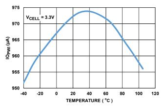
FIGURE 17. OPEN-WIRE TEST CURRENT vs TEMPERATURE (1mA SETTING)
