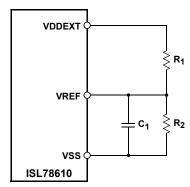
FIGURE 58. CELL READING ACCURACY ADJUSTMENT SYSTEM
