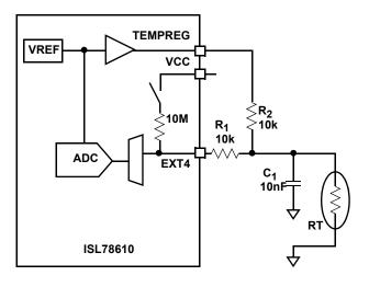
FIGURE 50. CONNECTION OF NTC THERMISTOR TO INPUT EXT4
