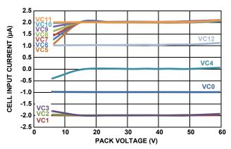
FIGURE 37. CELL INPUT CURRENT vs PACK VOLTAGE (+25°C)
