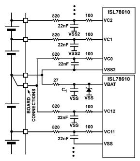
FIGURE 39. BATTERY CONNECTION BETWEEN STACKED DEVICES (OPTION 1)
