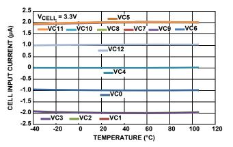
FIGURE 36. CELL INPUT CURRENT vs TEMPERATURE
