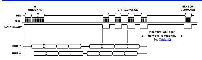
FIGURE 78. MINIMUM WAIT BETWEEN COMMANDS (DAISY CHAIN RESPONSE - TOP DEVICE)
