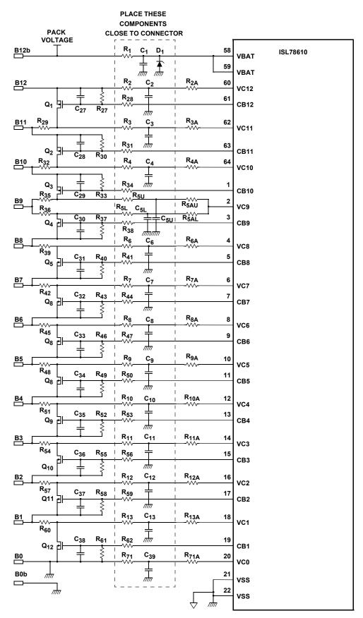
FIGURE 51. TYPICAL APPLICATIONS CIRCUIT - BATTERY CONNECTION CIRCUITS
