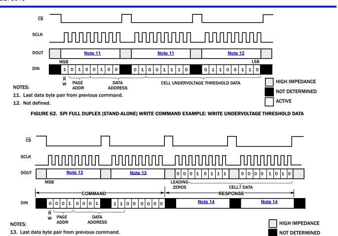
FIGURE 63. SPI FULL DUPLEX (STAND-ALONE) READ COMMAND EXAMPLE: READ CELL 7 DATA
