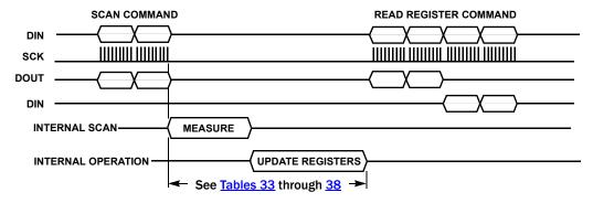
FIGURE 72. SCAN/MEASURE COMMAND TIMING WITH RESPONSE (STAND-ALONE)
