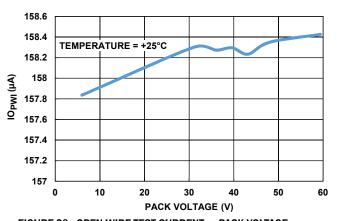
FIGURE 20. OPEN-WIRE TEST CURRENT vs PACK VOLTAGE (150 $\mu$ A SETTING)
