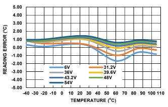
FIGURE 12. IC TEMPERATURE READING ERROR vs TEMPERATURE
