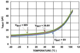
FIGURE 33. PACK VOLTAGE SHUTDOWN CURRENT vs TEMPERATURE (EN = 0) AT 6V, 39.6V, 60V
