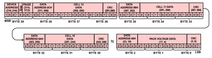
FIGURE 71D. DEVICE DATA RESPONSE: DEVICE 9, READ ALL CELL VOLTAGE DATA
