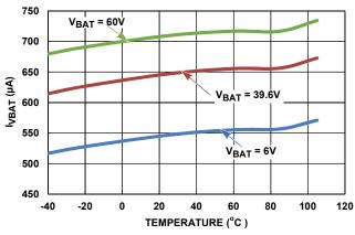
FIGURE 32. PACK VOLTAGE SUPPLY CURRENT VS TEMPERATURE AT 6V, 39.6V, 60V (DAISY CHAIN TOP)
