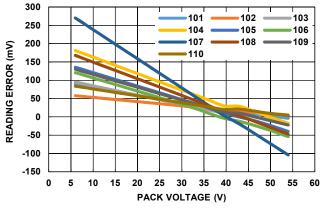
FIGURE 9. PACK VOLTAGE READING ERROR AT +25°C (MULTIPLE BOARDS)
