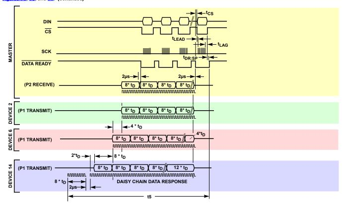
$$t5 \, = \, t_{SPI} \times 8 + t_{LEAD} + t_{LAG} + t_{DRSP} + t_{CS} + t_{D} \times (D \times 8 + 10 + N - 2) + 4 \mu s$$
