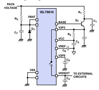
FIGURE 45. ISL78610 REGULATOR AND EXTERNAL CIRCUIT SUPPLY ARRANGEMENT
