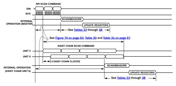
FIGURE 73. MEASUREMENT TIMING (6 DEVICE DAISY CHAIN)
