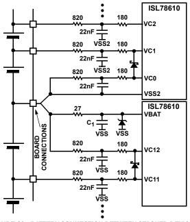
FIGURE 40. BATTERY CONNECTION BETWEEN STACKED DEVICES (OPTION 2)
