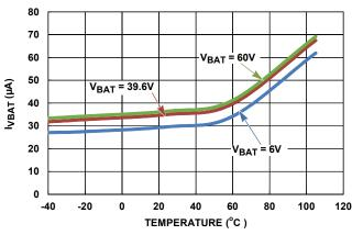
FIGURE 26. PACK VOLTAGE SLEEP CURRENT VS TEMPERATURE AT 6V, 39.6V, 60V (DAISY CHAIN MASTER)
