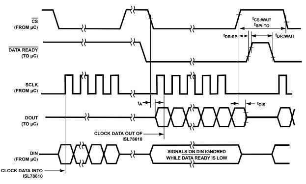
FIGURE 4. SPI HALF DUPLEX (3-WIRE) INTERFACE TIMING
