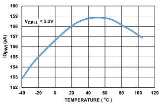
FIGURE 19. OPEN-WIRE TEST CURRENT VS TEMPERATURE (150µA SETTING)
