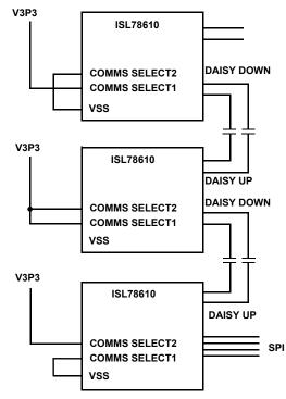
FIGURE 47. DAISY CHAIN COMMUNICATIONS CONNECTIONS AND SELECTION
