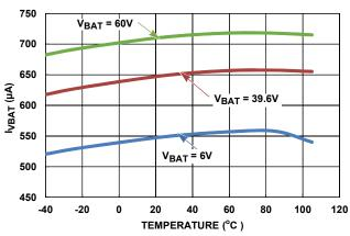
FIGURE 30. PACK VOLTAGE SUPPLY CURRENT vs TEMPERATURE AT 6V, 39.6V, 60V (DAISY CHAIN MASTER)
