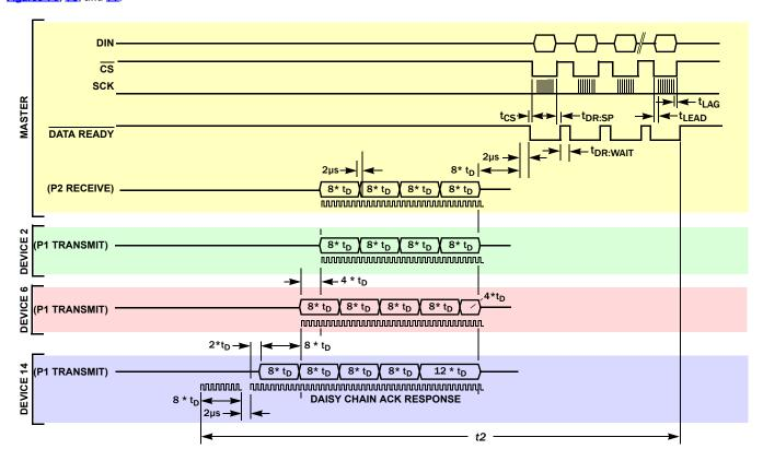
$$t2 = (8 \times t_{SPI} + t_{DRSP} + t_{DRWAIT} + t_{CS} + t_{LEAD} + t_{LAG}) \times D - t_{DRSP} + t_{D} \times (42 + N - 2 + 8) + 4 \mu s$$
