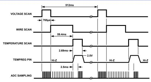
FIGURE 59. SCAN TIMING EXAMPLE DURING SCAN CONTINUOUS MODE AND SCAN ALL MODE
