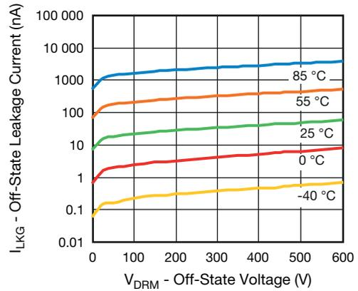
Fig. 7 - Off-State Leakage Current vs. Off-State Voltage
