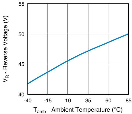
Fig. 5 - Reverse Voltage vs. Ambient Temperature
