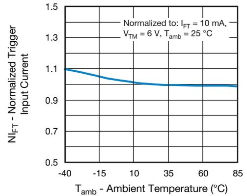
Fig. 8 - Normalized Trigger Input Current vs. Ambient Temperature
