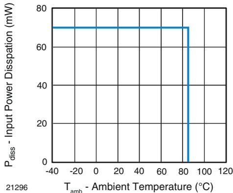
Fig. 1 - Input Power Dissipation vs. Ambient Temperature
