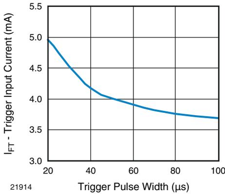
Fig. 11 - Trigger Input Current vs. Trigger Pulse Width
