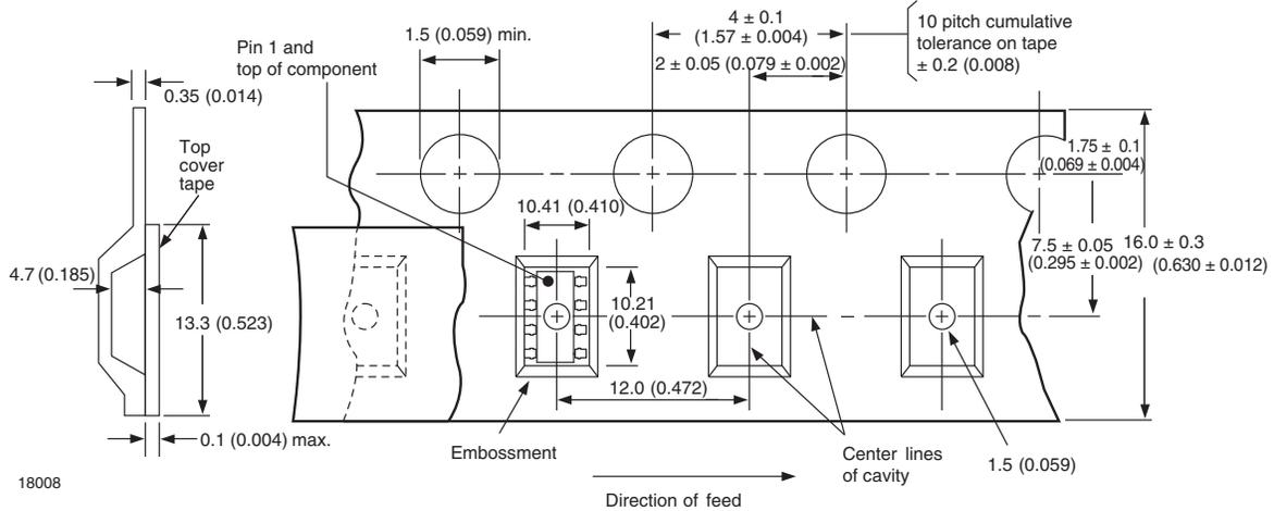
Fig. 16 - Tape and Packing (1000 pieces on reel)
