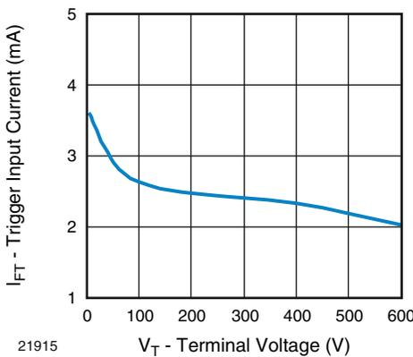
Fig. 12 - Trigger Input Current vs. Terminal Voltage
