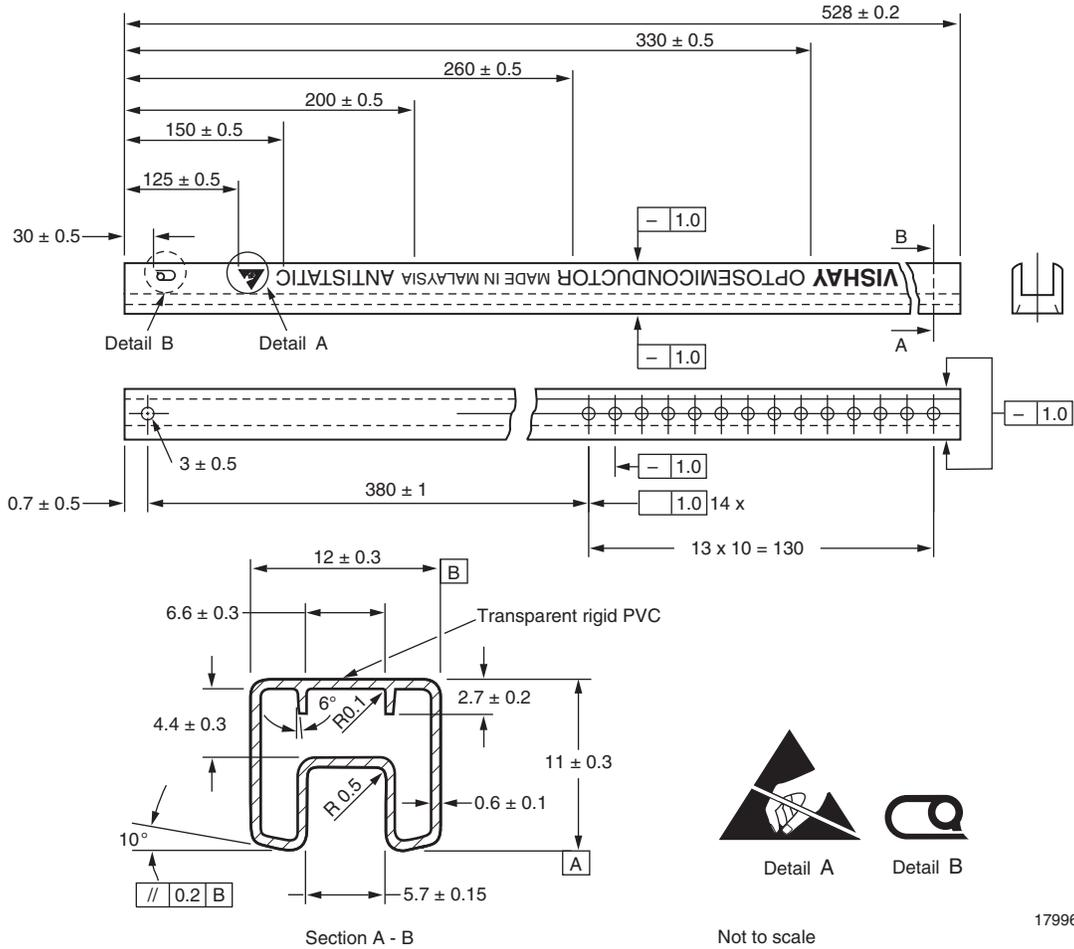
Fig. 13 - Shipping Tube Specifications for DIP Packages
