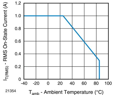
Fig. 2 - RMS On-State Current vs. Ambient Temperature
