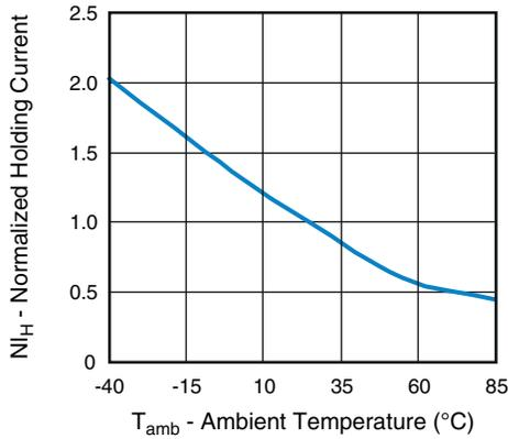
Fig. 10 - Normalized Holding Current vs. Ambient Temperature
