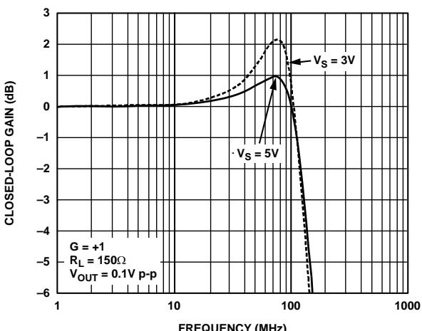
Figure 7. Small Signal Frequency Response for Various Supplies
