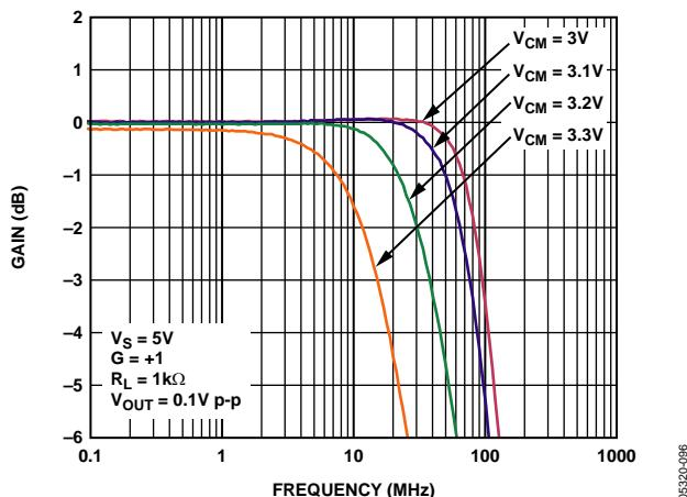
Figure 38. Unity-Gain Follower Bandwidth vs. Frequency for Various Input Common-Mode
