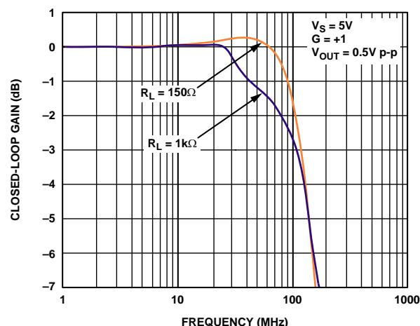
Figure 10. Large Frequency Response for Various Loads
