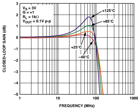
Figure 11. Small Signal Frequency Response for Various Temperatures
