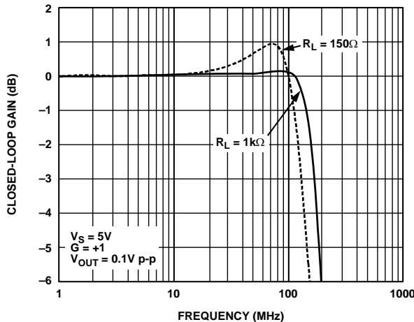
Figure 6. Small Signal Frequency Response for Various Loads
