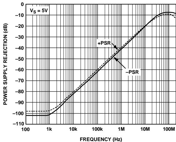
Figure 35. Power Supply Rejection (PSR) vs. Frequency
