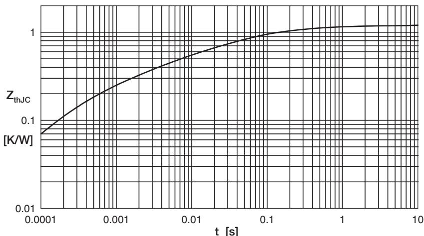
Fig. 7 Transient thermal impedance junction to case
