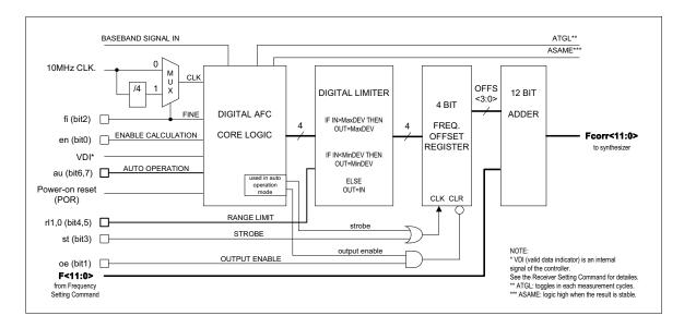
In automatic operation mode (no strobe signal is needed from the microcontroller to update the output offset register), the AFC circuit is automatically enabled when VDI indicates a potential incoming signal during the whole measurement cycle and the circuit measures the same result in two subsequent cycles.
