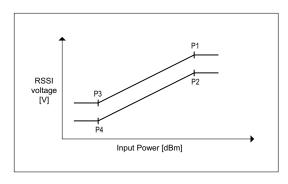
Voltage on ARRSI pin vs. Input RF power
