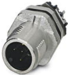
Sensor/actuator flush-type connector, connector, 5-pos., M12 SPEEDCON, shielded, A-coded, rear/screw mounting with M12 thread, with straight THR solder connection
