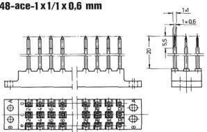
Remaining dimensions as for wiring strip VE 48-ace-1 x 1
