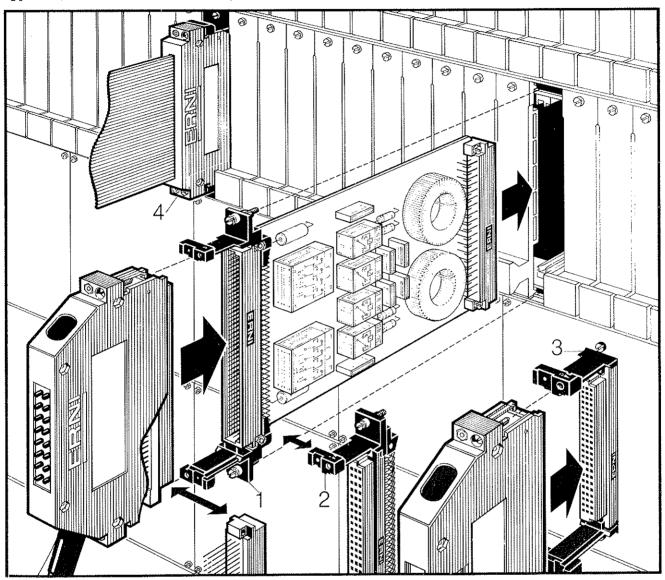
This interface system gives users the opportunity of providing mateable connections on the front-panels. The guide elements can either be fitted as pull grips or be mounted on metal front panels.
