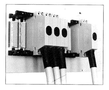
A particular advantage of this method of interconnection wiring is the wide variety of wiring methods that are possible. A female connector type chosen to suit the wiring method used (wire wrapping, solder, fast-on or piggy-back connections) is fitted in the interconnection field.
