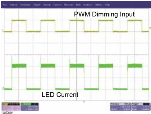
(a) PWM Dimming Performance Time Scale : 1ms/div
