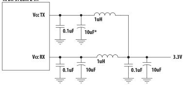
Note: Inductors should have less than 1 Ohm series resistor per MSA \* optional capacitance but recommended (required for SFP+)
