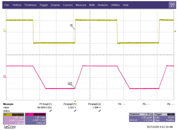
Figure 10. Non-Inverting Large Signal Step Response
