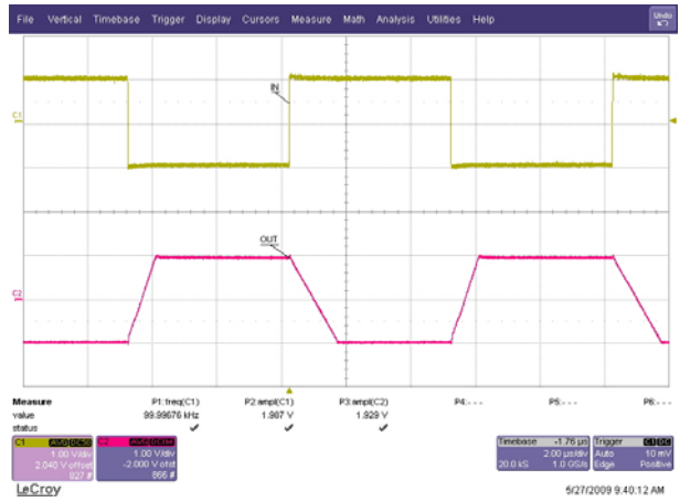
Figure 12. Inverting Large Signal Step Response
