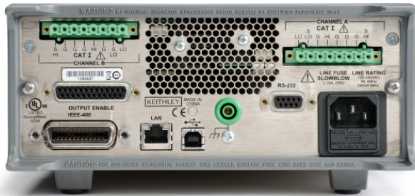
Model 2604B/2614B rear panel (Single channels 2601B, 2611B, 2635B not shown)
