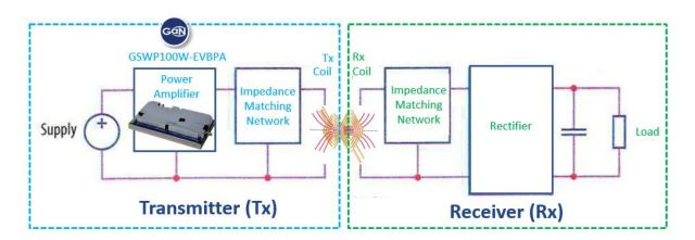
Figure 1 - A magnetic resonant wireless power transfer design.
