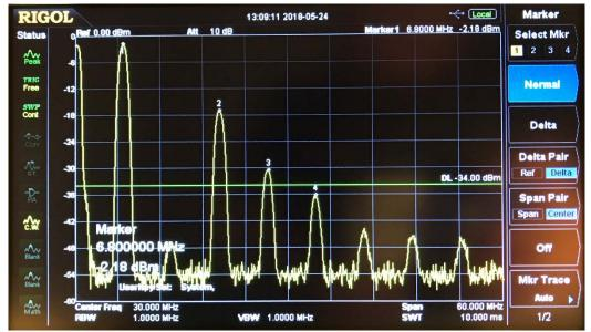
Figure 19 • Spectrum Plot of output terminal JP56 SMA after 49.66dB attenuation at 100W output power
