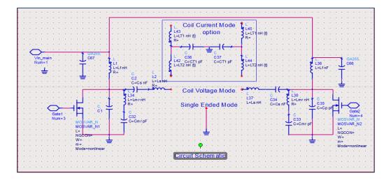
Figure 6 • GSWP100W-EVBPA WPT Class EF2 PA Block Diagram
