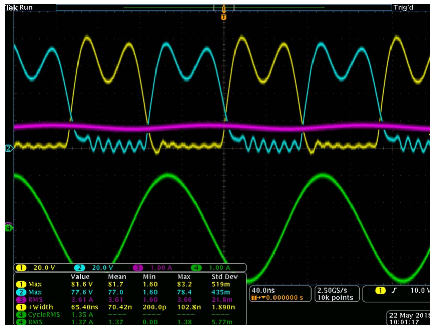
Figure 18 • Oscilloscope Plot Showing Both GS61008P Drain Node Signals
