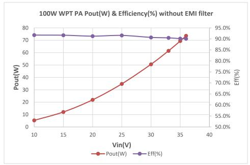
**Figure 20 •** Output power and efficiency of PA without EMI filter at JP56 SMA Note: With the EMI filter, the maximum power level is limited to 80W, due to the  $50\Omega$  test.
