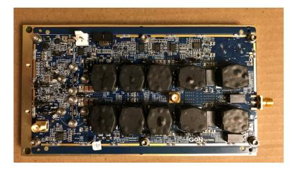
Figure 2 • Top side of GSWP100W-EVBPA Evaluation Board Assembly
