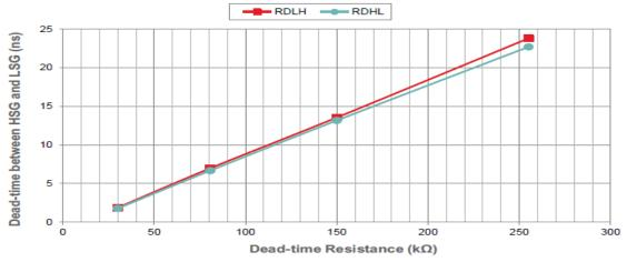
Figure 9 • Dead Time vs Dead Time Resistor
