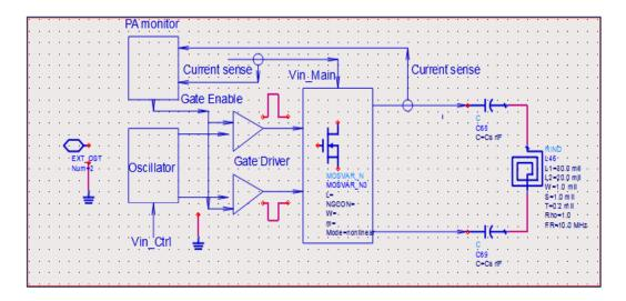
Figure 5 • GSWP100W-EVBPA WPT Push-Pull EVB Block Diagram
