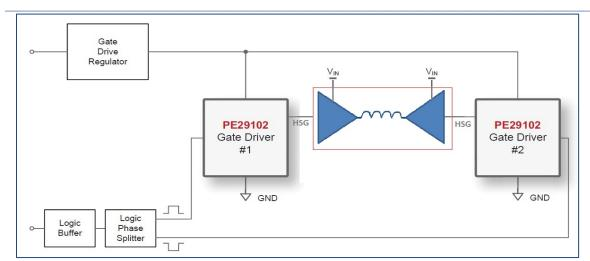
Figure 7 • GSWP100W-EVBPA WPT driver Block Diagram
