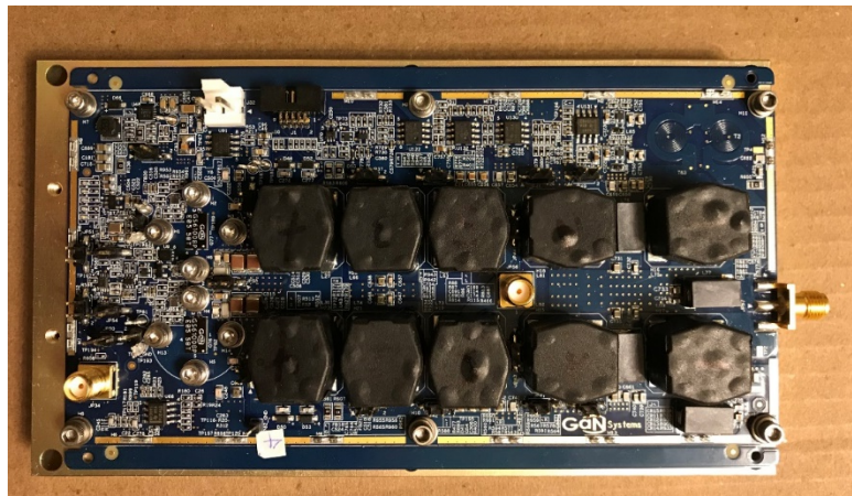
Figure 2 • Top side of GSWP100W-EVBPA Evaluation Board Assembly
