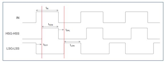
Figure 8 • PE29102 Dead-time Waveforms and Duty Cycle Setting
