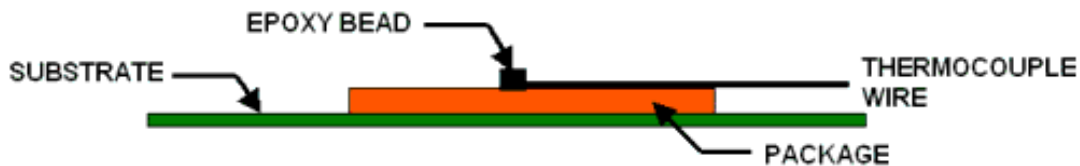
Figure 13-7 Technique for Measuring T_{case} with 0° Angle Attachment, No Heatsink
