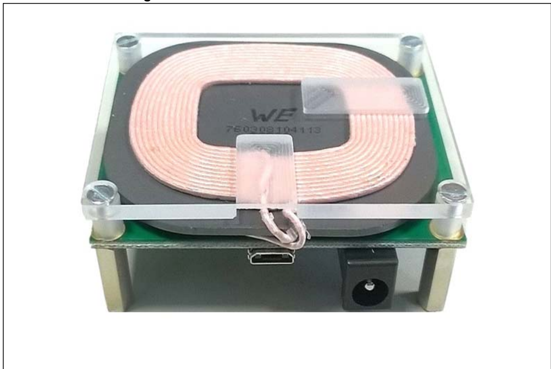
Figure 3. STEVAL-ISB044V1 evaluation board
