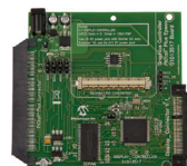
Graphics Controller PICtail™ Plus Epson S1D13517 Board (AC164127-7)
