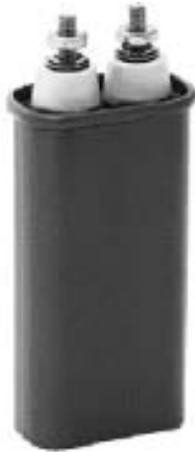
Type T capacitors are for high voltage filter applications as well as being used for filtering, bypass and blocking in radar amplifiers and power supplies. The Type T is constructed with a rugged inserted tab to foil connection to 10-32 screw terminals surrounded by thermoset plastic bushings for high voltage performance in an oval, hermetically sealed metal case that will give long operating life under harsh conditions.
