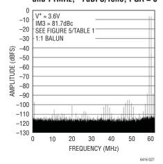
LTC6416 Driving LTC2208 16-Bit ADC, 64K Point FFT,  $f_{IN} = 139.5$ MHz and 140.5MHz, -7dBFS/Tone, PGA = 0
