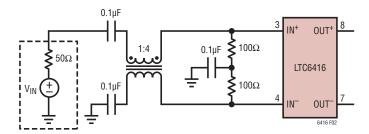
Figure 2. Input Termination for Differential  $50\Omega$  Input Impedance Using a 1:4 Balun
