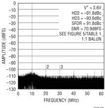
LTC6416 Driving LTC2208 16-Bit ADC, 64K Point FFT,  $f_{\text{IN}} = 30\text{MHz}$  and 31MHz, -7dBFS/Tone, PGA = 0
