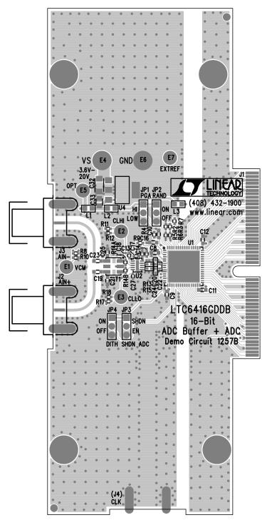
Figure 8. Demo Board DC1257B Layout
