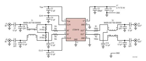
Figure 7. Demo Board DC1287A Schematic (Test Circuit A)
