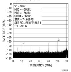
LTC6416 Driving LTC2208 16-Bit ADC, 64K Point FFT, f<sub>IN</sub> = 70MHz, -1dBFS, PGA = 1
