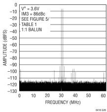
LTC6416 Driving LTC2208 16-Bit ADC, 64K Point FFT, f<sub>IN</sub> = 70MHz and 71MHz, -7dBFS/Tone, PGA = 0
