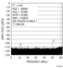
LTC6416 Driving LTC2208 16-Bit ADC, 64K Point FFT, f<sub>IN</sub> = 140MHz, -1dBFS, PGA = 0
