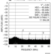
LTC6416 Driving LTC2208 16-Bit ADC, 64K Point FFT,  $f_{IN} = 140 MHz$ , -1dBFS, PGA = 1
