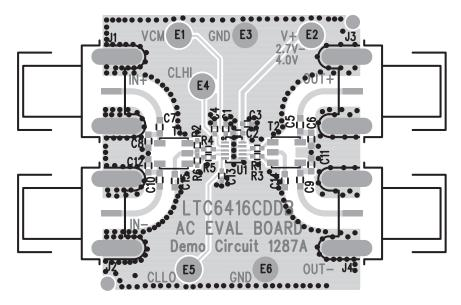
Figure 6. Demo Board DC1287A Layout
