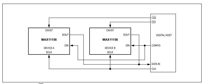
Figure 10. Multichannel CS Configuration Diagram
