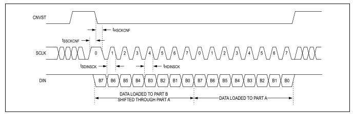
Figure 5. Input Configuration Timing in Daisy-Chain Mode
