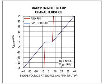
Figure 1. Input Clamp Characteristics
