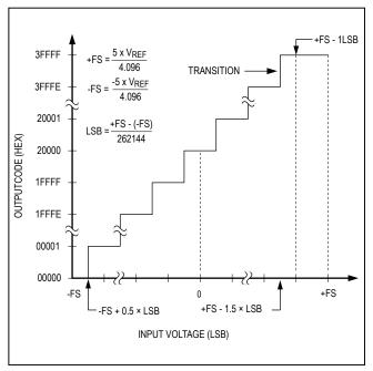
Figure 3. Bipolar Transfer Function
