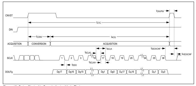
Figure 13. Daisy-Chain, No-Busy Indicator Mode Timing
