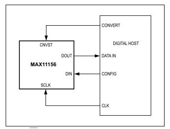
Figure 6. CS No-Busy Indicator Mode Connection Diagram
