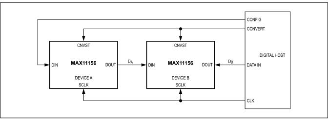
Figure 12. Daisy-Chain, No-Busy Indicator Mode Connection Diagram
