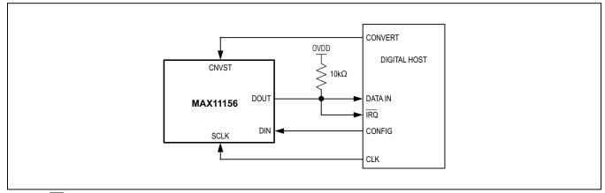
Figure 8. CS With Busy Indicator Mode Connection Diagram
