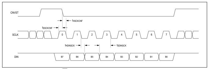
Figure 4. Input Configuration Timing in CS Mode
