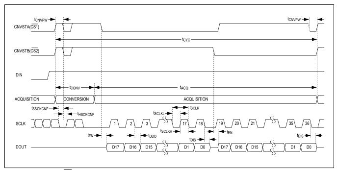
Figure 11. Multichannel CS Configuration Timing
