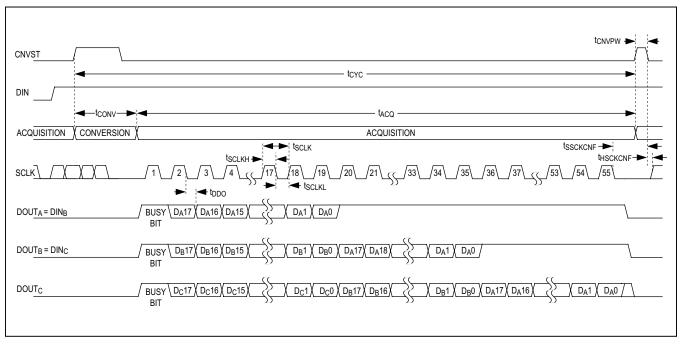
Figure 15. Daisy-Chain Mode with Busy Indicator Timing
