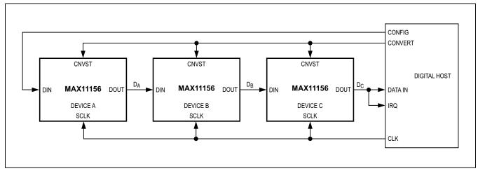
Figure 14. Daisy-Chain Mode with Busy Indicator Connection Diagram
