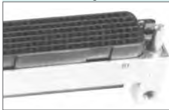
Chevron Grid - Up to 300 Contacts in 6 Rows.
