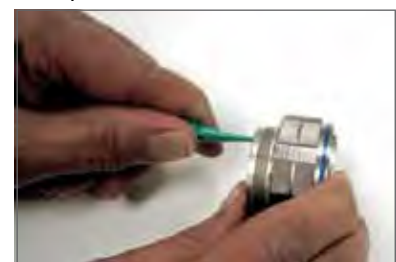
Plastic tool with contact in proper position.
