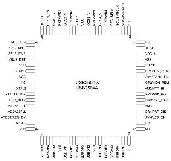
Figure 3.1 4-Port 64 Pin TQFP
