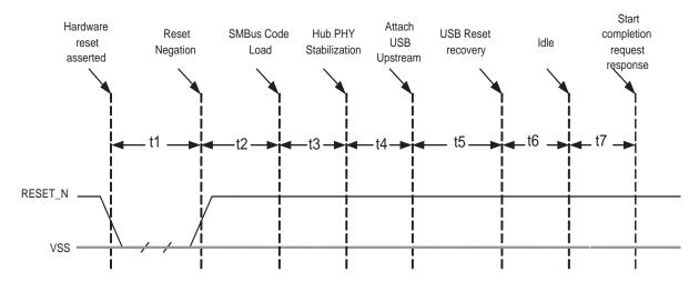
Figure 5.4 Reset\_N Timing for SMBus Mode
