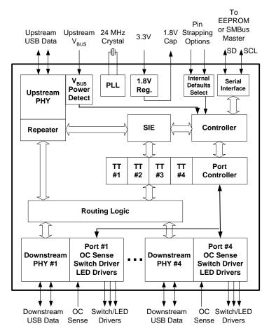
Figure 4.1 4-Port Block Diagram
