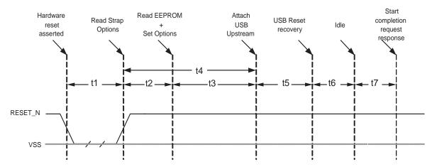
Figure 5.3 Reset\_N Timing for EEPROM Mode
