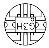
MARKING FOR PIN1 IS ON TOP OF CHIP
