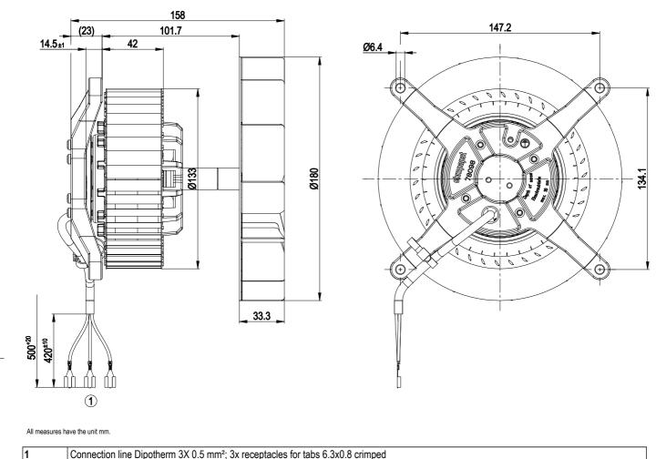
Connection line Dipotherm 3X 0.5 mm<sup>2</sup>; 3x receptacles for tabs 6.3x0.8 crimped
