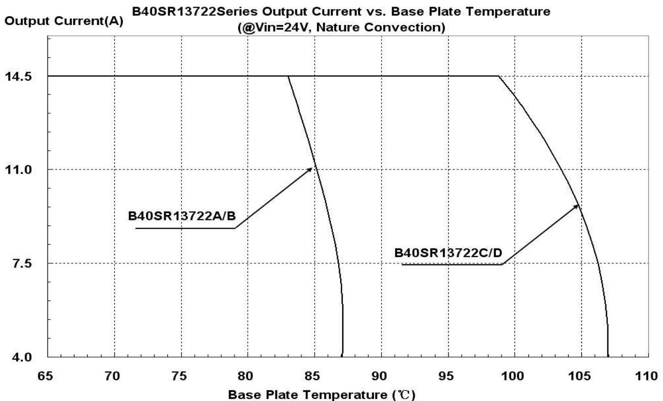
Figure 21: Output Current vs. Base Plate temperature @Vin=24V
