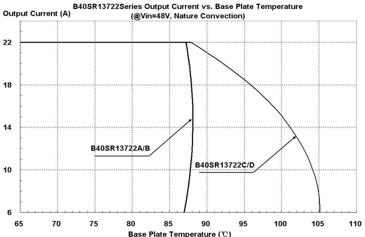
Figure 23: Output Current vs. Base Table temperature @ Vin=48V
