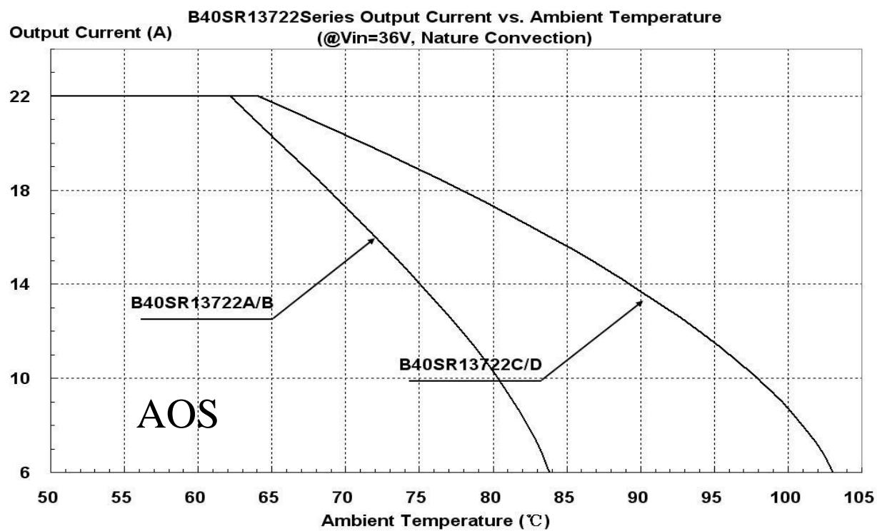
**Figure 18:** Output Current vs. Ambient temperature @ Vin=36V
