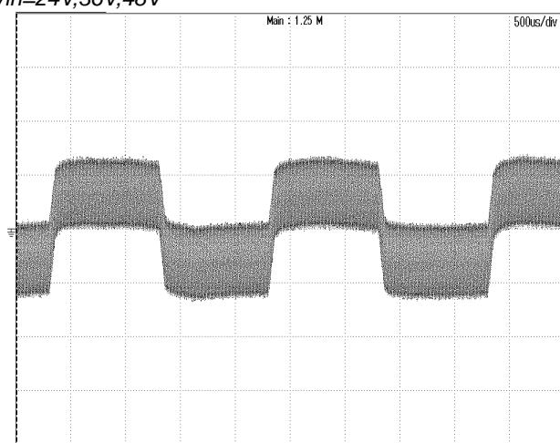
**Figure 3:** Dynamic response to load step 11A~16.5A with 0.1A/uS slew rate at 48Vin
