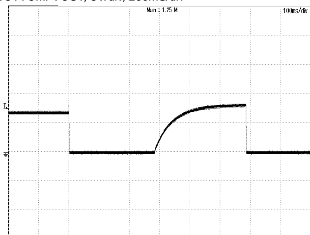
Figure 4: Vout start up with Vin on at 48Vin,22A Iout, TOP:VIN, 20V/div, 200mS/div BOTTOM: VOUT, 5V/div, 200mS/div
