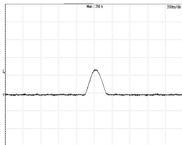
**Figure 11:** Inrush current @ Vin=48V
