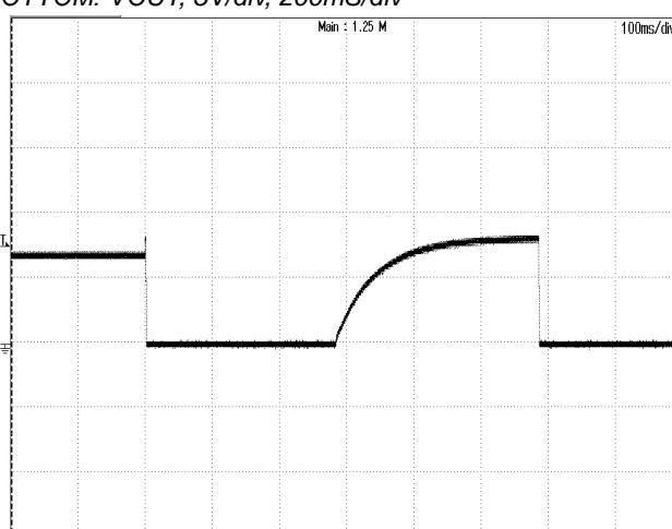
**Figure 6:** Output over voltage protection at 48Vin, 22A lout
