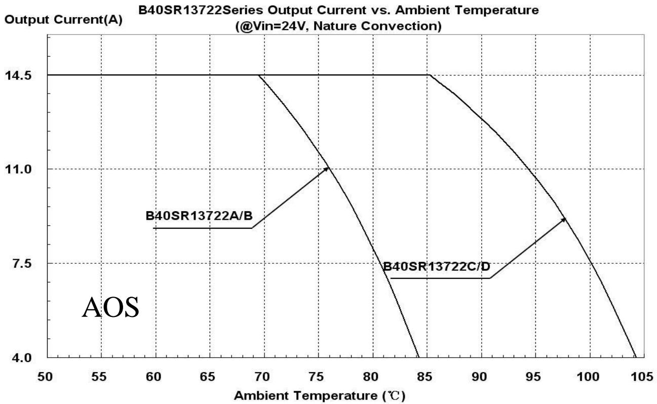
Figure 17: Output Current vs. Ambient temperature @Vin=24V
