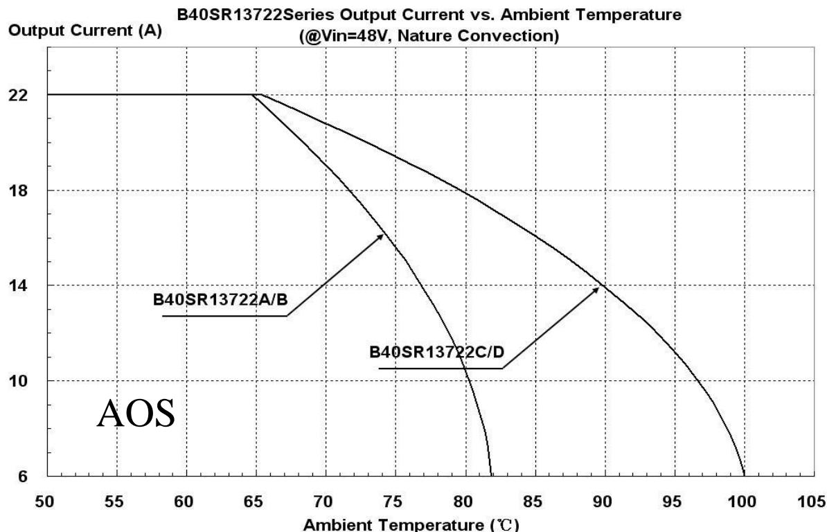
**Figure 19:** Output Current vs. Ambient temperature @ Vin=48V
