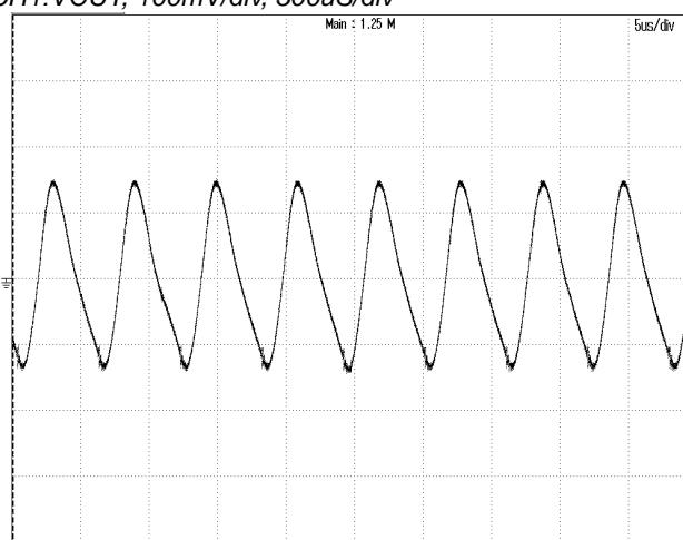
**Figure 5:** Output ripple & noise at 48Vin, 22A lout
