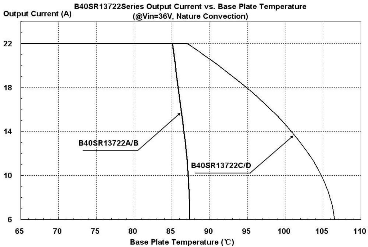
Figure 22: Output Current vs. Base Table temperature @ Vin=36V
