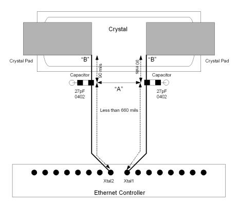
Figure 51. Recommended Crystal Placement and Layout
