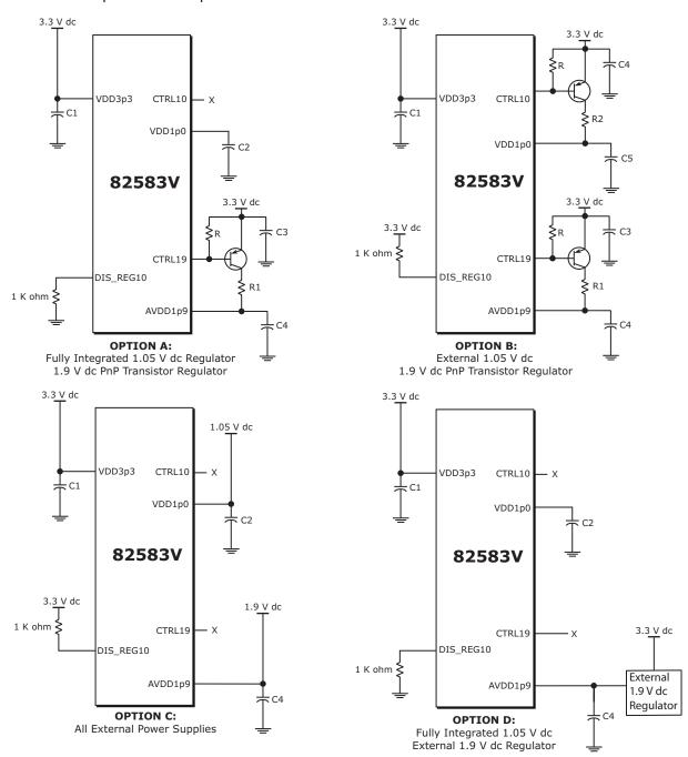
Figure 4. Power Scheme Schematics
