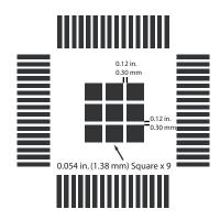
Figure 63. 82583V Solder Paste
