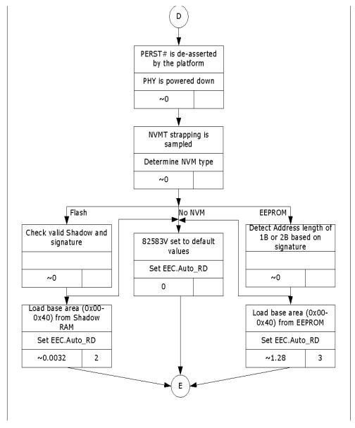
Figure 13. 82583V Initialization - NVM Load After PE\_RST\_N
