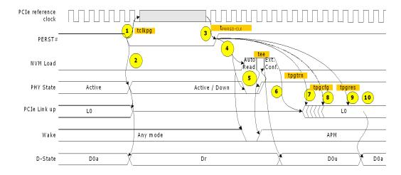
Figure 18. Global Reset Timing Diagram
