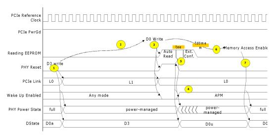
Figure 41. D3hot Transition Timing Diagram
