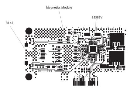
Figure 56. Layout for Discrete Magnetics
