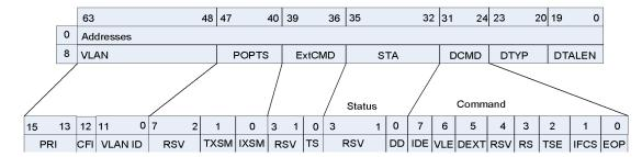
Figure 37. Extended Data Descriptor Format
