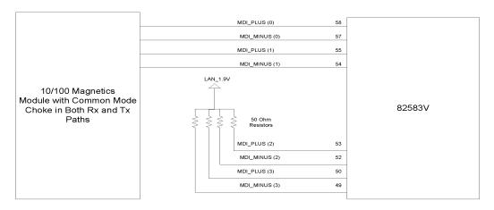
Figure 54. 82583V 10/100 Mb/s Magnetics Module Connections (With CMC)
