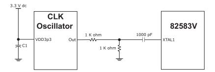
Figure 52. Oscillator Solution
