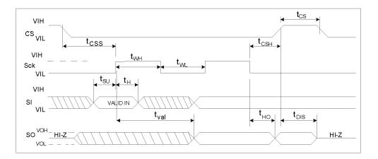
Figure 5. Flash Timing Diagram
