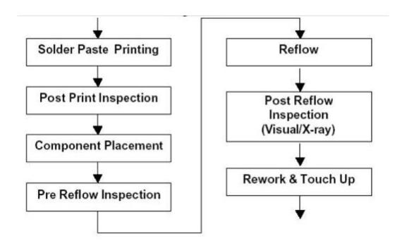
Figure 66. Assembly Flow
