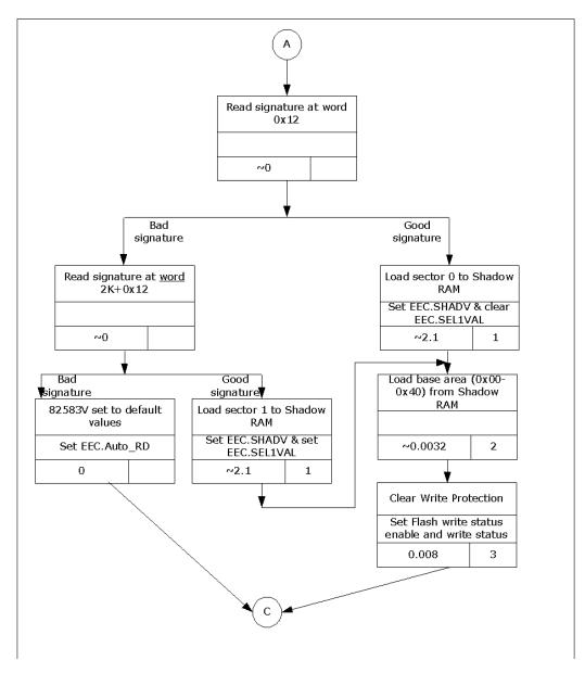
Figure 10. 82583V Initialization - Flash Load
