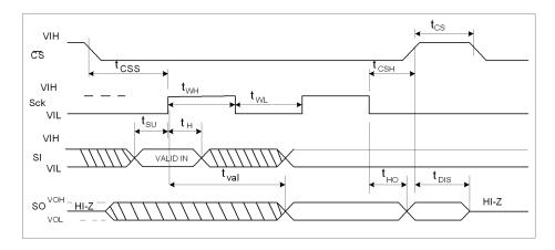
Figure 6. **EEPROM Timing Diagram**
