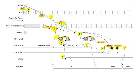
Figure 15. Power-Up Timing Diagram
