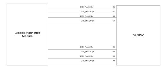
Figure 53. 82583V Gigabit Magnetics Module Connections
