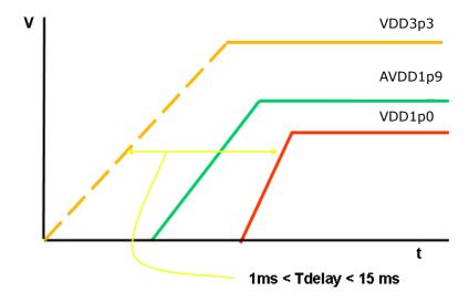
Figure 60. Internal LVR Power-Up Sequence
