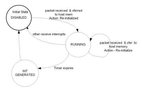
Figure 31. Packet Delay Timer Operation (With State Diagram)
