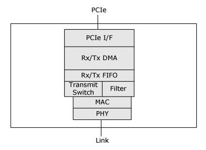
Figure 1. 82583V Architecture Block Diagram
