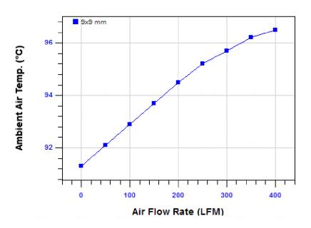
Figure 70. Maximum Allowable Ambient Temperature vs. Air Flow
