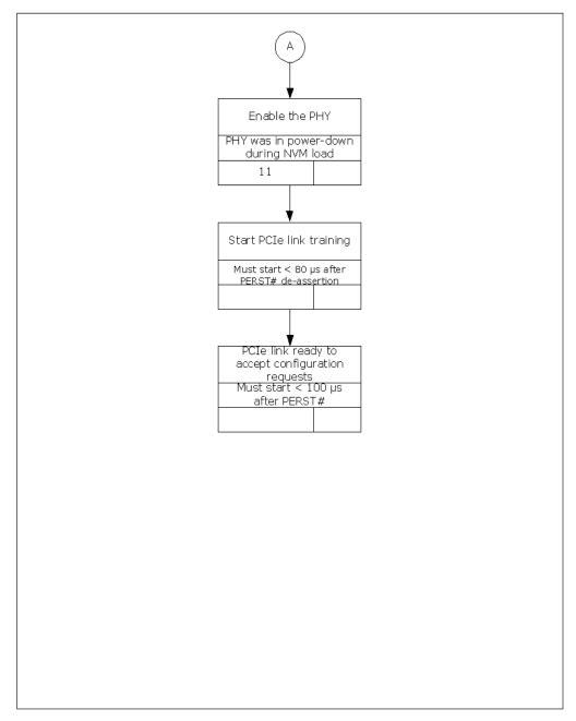
Figure 17. 82583V Global Reset - PHY and PCIe
