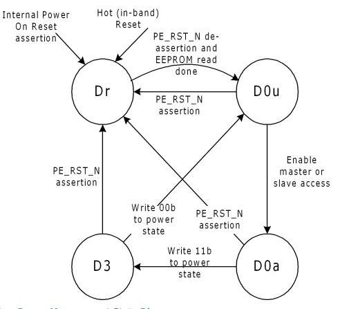
Figure 40. Power Management State Diagram
