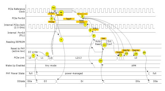
Figure 42. D3cold Transition Timing Diagram
