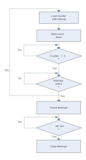
Figure 39. Interrupt Throttle Flow Diagram
