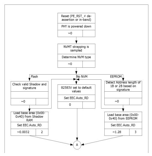
Figure 16. 82583V Global Reset - NVM Load
