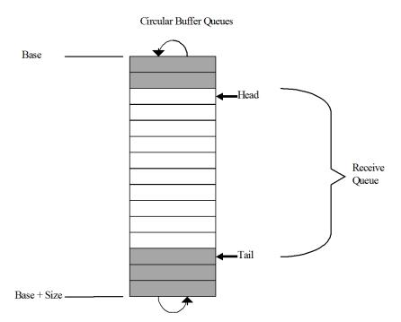
Figure 30. Receive Descriptor Ring Structure
