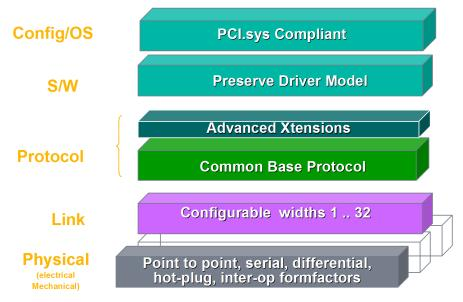
Figure 23. PCIe Stack Structure
