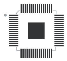
Figure 61. 82583V Silkscreen and Components Pad (Top View)
