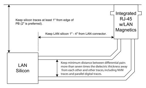
**Note:** Figure 55 represents a 10/100 diagram. Use the same design considerations for the two differential pairs not shown for gigabit implementations.
