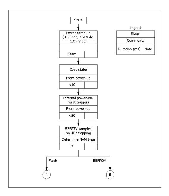
Figure 9. 82583V Initialization - Power-On Reset
