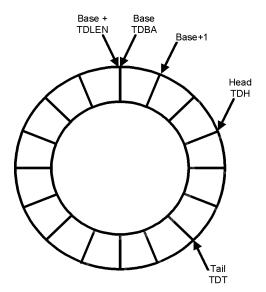
Figure 33. Transmit Descriptor Ring Structure
