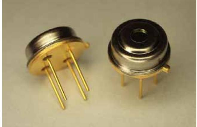
This thermopile sensor is used for non-contact surface temperature measuring. The ZTP -101T model consists of thermo-elements, flat IR filter, a thermistor for temperature compensation and a hermetically-sealed small-size package. There is also a variety of filters available to maximize performance in specific applications
