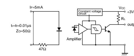
Fig.8 Response time measurement circuit
