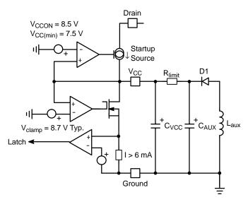
Figure 34. A more detailed view of the NCP1027 offers better insight on how to properly wire an auxiliary winding.
