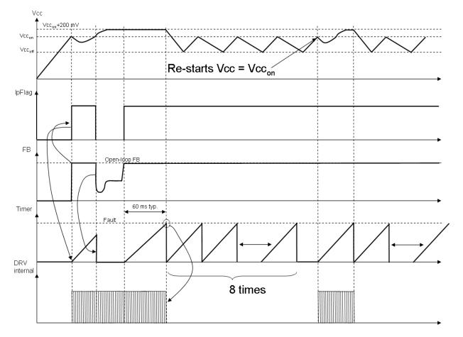
Figure 27. In case of short–circuit or overload, the NCP1027 protects itself and the power supply via a low frequency burst mode. The V<sub>CC</sub> is maintained by the current source and self–supplies the controller.
