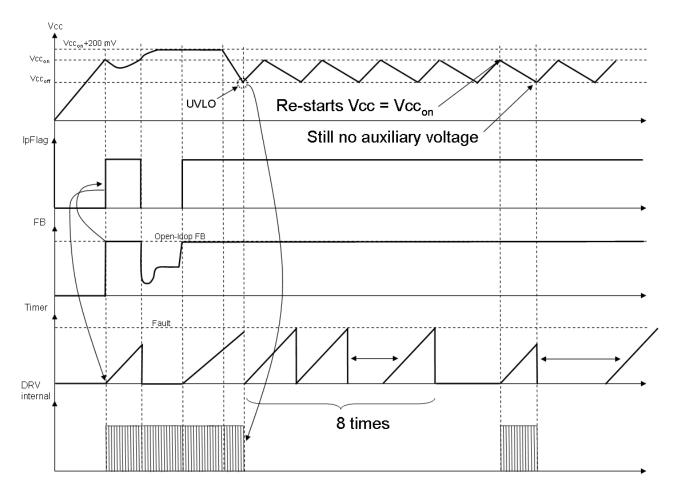
Figure 28. The auxiliary winding collapses in presence of a short-circuit. Pulses are immediately stopped as  $V_{CC}$  crosses the minimum operating voltage,  $VCC_{(min)}$ .
