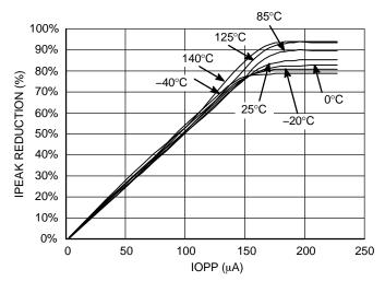
Figure 23. Ipeak Reduction = F(lopp, @ temperature)
