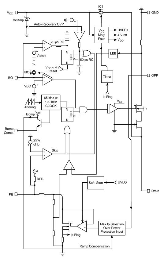
Figure 2. Internal Block Diagram
