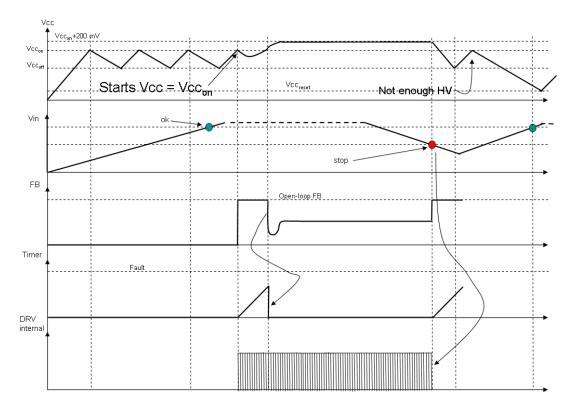
Figure 31. Signal Evolution During a Brown-Out Condition
