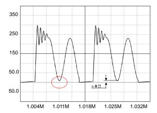
Figure 45. The reflected voltage shall always be greater than the minimum input voltage to avoid the forward biasing of the MOSFET body-diode.
