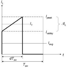
Figure 46. Primary Inductance Current Evolution in CCM
