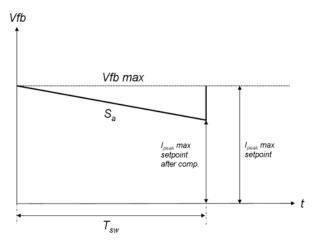
Figure 41. Maximum Peak Current Setpoint Variations versus Ramp Compensation
