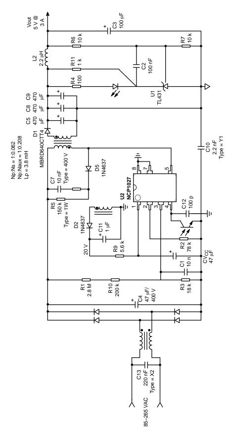
Figure 49. 5.0 V-3.0 A Universal Mains Power Supply
