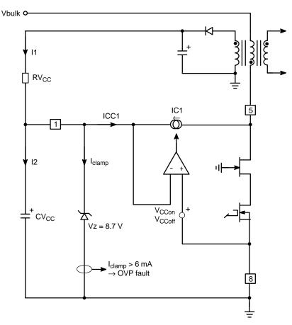
Figure 24. Internal Arrangement of the Startup Circuitry
