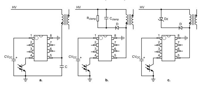
Figure 47. Different Options to Clamp the Leakage Spike
