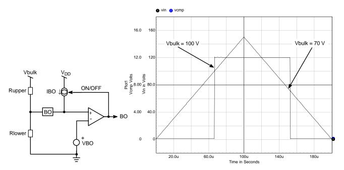
Figure 30a. The internal brown-out configuration with an offset current source.
