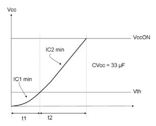
Figure 26. The startup source now features a dual-level startup current.
