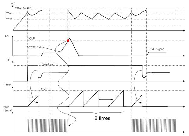
Figure 36. If the V<sub>CC</sub> current exceeds a certain threshold, an auto-recovery protection is activated and protects the design.
