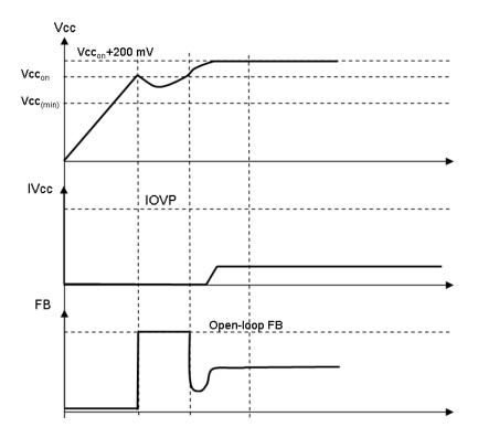
Figure 25. A typical startup sequence showing the V<sub>CC</sub> capacitor voltage evolution versus time.
