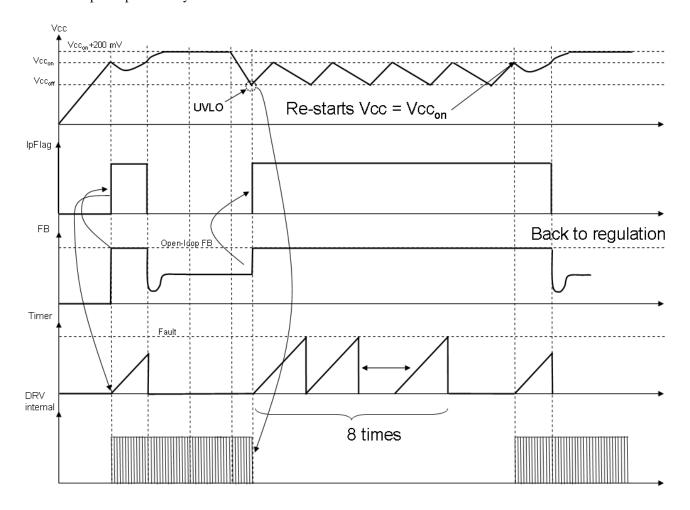
Figure 29. In this particular case, the output goes low but the timer is not started since the FB pin is still held by the optocoupler. Due to the UVLO circuit, the controller safely stops operation at  $V_{CC} = VCC_{(min)}$ .
