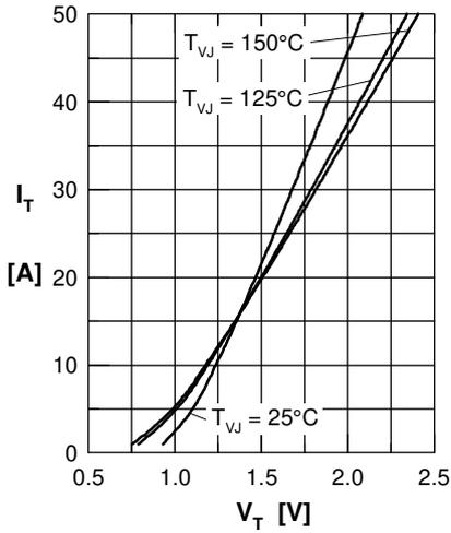
Fig. 1 Forward characteristics
