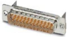
D-SUB contact insert, shell size 3, with 25 signal contacts, contact type pin, for PCB assembly, angled, fixing with a 2.5 mm hole and solder metal plate, for panel mounting frame VS-25-...
