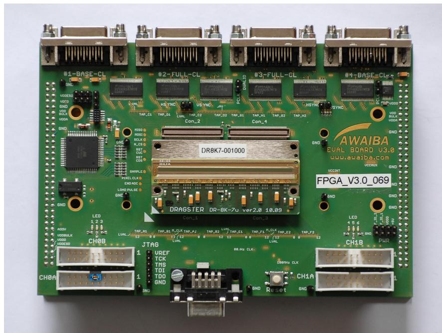
Figure 5: Assembling DR\_8K\_7um on the Evaluation Board
