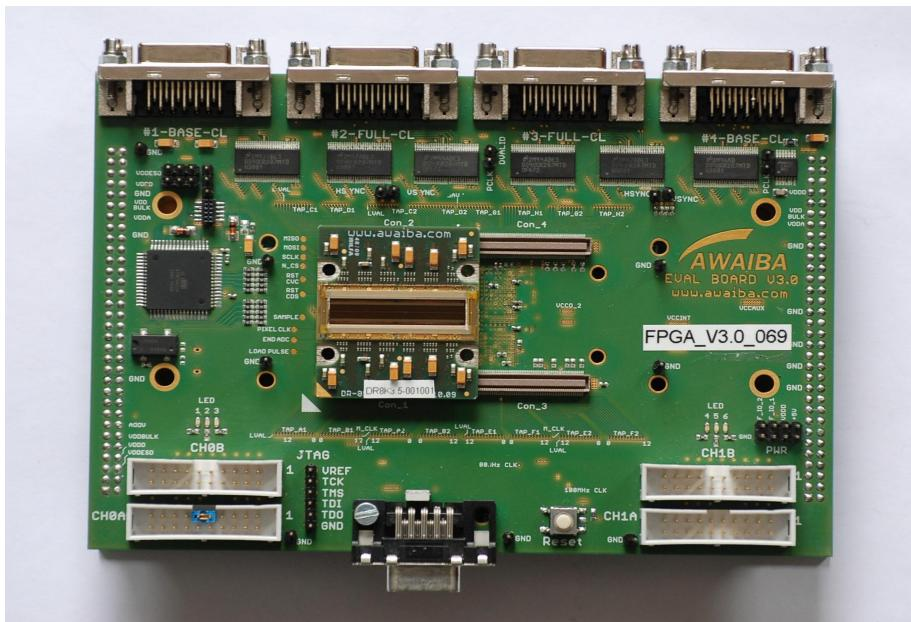
Figure 8: Assembling DR\_8K\_3.5um on the Evaluation board
