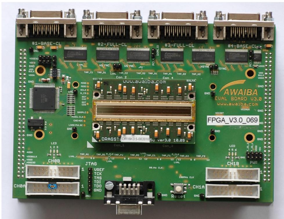
Figure 9: Assembling DR\_16K\_3.5um on the Evaluation Board
