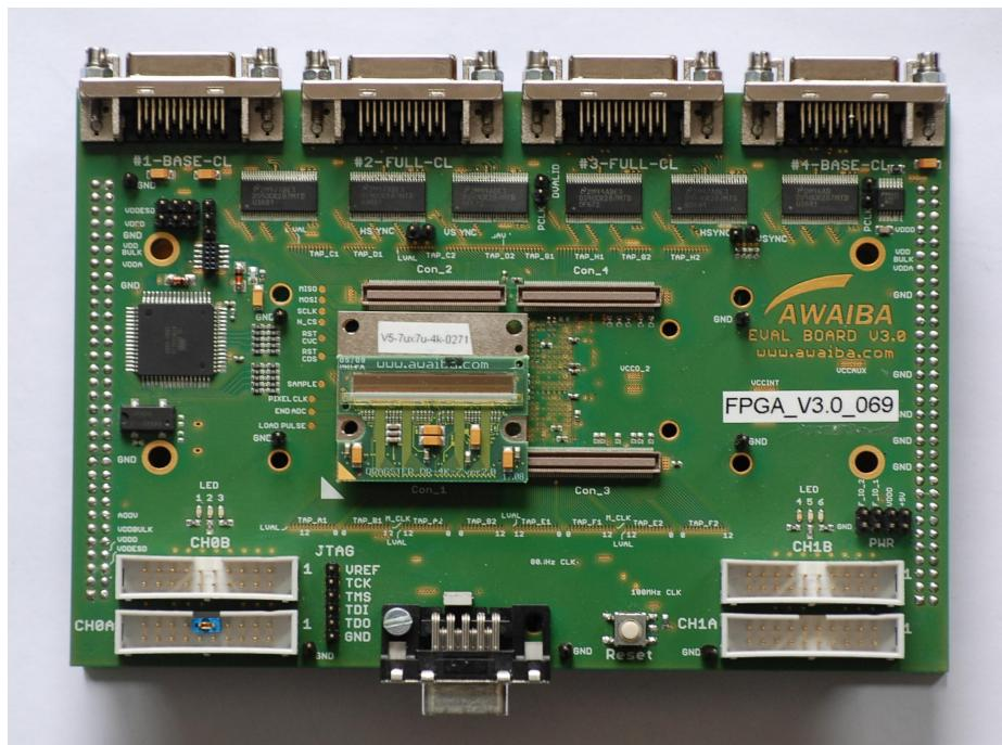
Figure 4: Assembling DR\_4K\_7um on the Evaluation board
