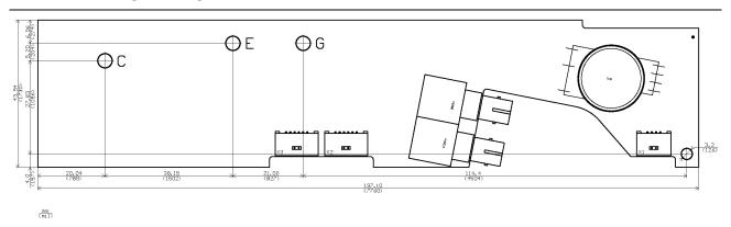
Maximum driver height: 13mm measured from the bottom layer
