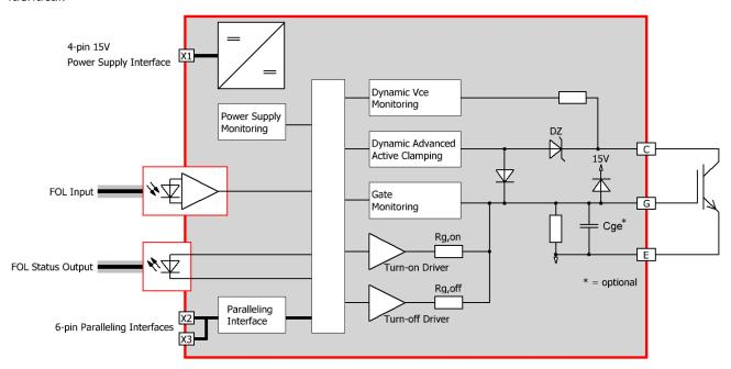
Fig. 2 Basic schematic of the 1SP0635V and 1SP0635S drivers
