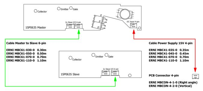
Fig. 11 Cable arrangement for 1SP0635 (Master only or Master and Slave)
