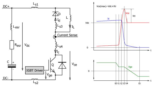
Fig. 22 Test circuit (left) and typical switching behavior (right)
