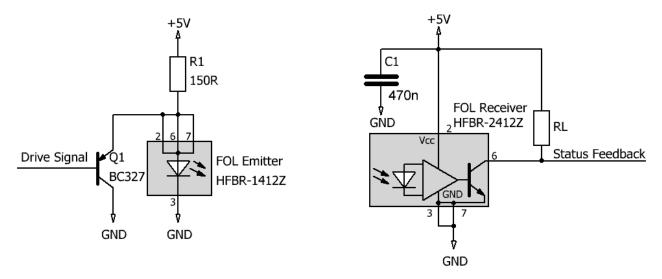
Fig. 18 Recommended circuitry for the "ST" fiber-optic links (1SP0635S)
