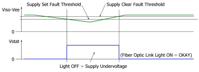
Fig. 16 Status feedback in the event of a supply undervoltage of the master driver
