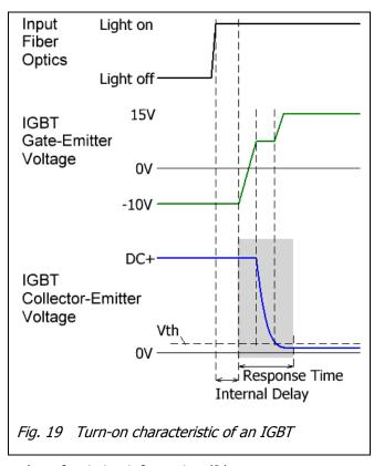
A dynamic  $V_{Ce}$  monitoring circuit is implemented in 1SP0635V and 1SP0635S gate drivers. The IGBT collector-emitter voltage is measured with a resistor network.
