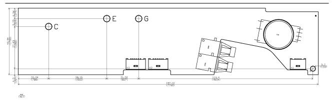
Maximum driver height: 12mm measured from the bottom layer
