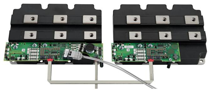
Fig. 1 1SP0635V (master, left) with 1SP0635D (slave, right) each screwed onto a 3.3kV IGBT module
