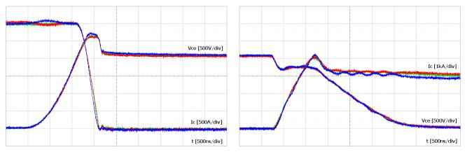
Fig. 21 Turn-off (left) and turn-on (right) behavior of three 1500A/3300V IGBT modules in parallel connection at a DC-link voltage of 2200V and a collector current of 3000A each
