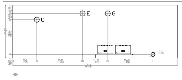
Maximum driver height: 6mm measured from the bottom layer
