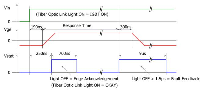
Fig. 14 Driver behavior and status feedback in the short-circuit condition
