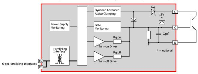
Fig. 3 Basic schematic of the 1SP0635D drivers
