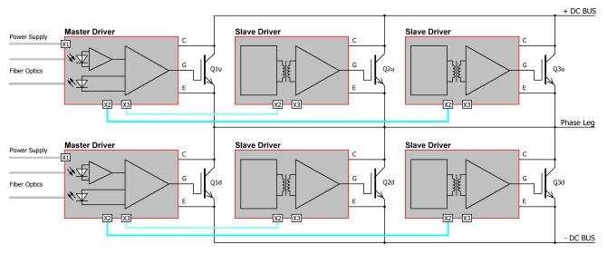
Fig. 4 Principle of parallel connection of 1SP0635 drivers with one master and two slaves in a half-bridge configuration (example)
