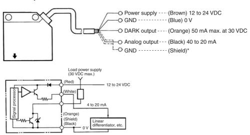
Note: \*The two ground terminals (black and shield) are internally connected. However, the black ground must be used with the red terminal for the power supply and the shield ground must be used with the white terminal for the analog output.
