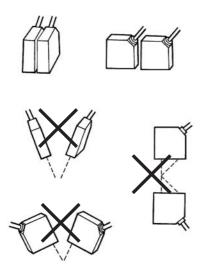
When using the LED Displacement Sensor in combination with another type of Sensor (such as a Photoelectric Sensor), the sensor beams should be as close to perpendicular as possible.
