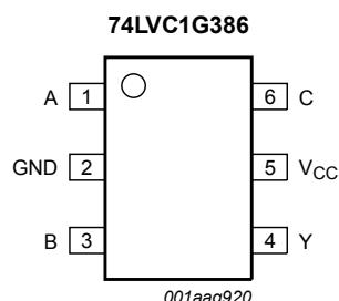
Figure 4. Pin configuration
