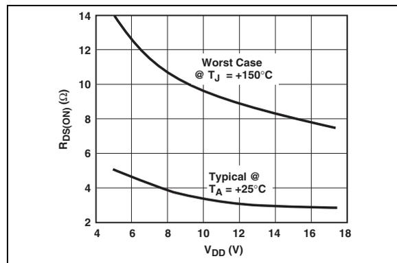
**FIGURE 2-12:** Output Resistance (Output Low) vs. Supply Voltage.
