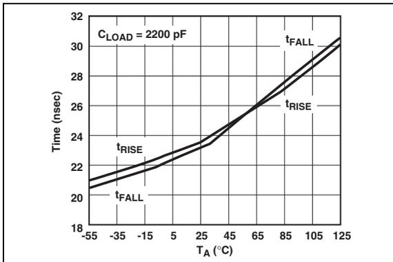
**FIGURE 2-3:** Rise and Fall Times vs. Temperature.
