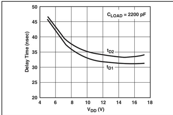
**FIGURE 2-7:** Propagation Delay Time vs. Supply Voltage.
