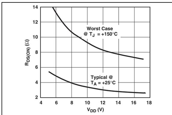
**FIGURE 2-9:** Output Resistance (Output High) vs. Supply Voltage.
