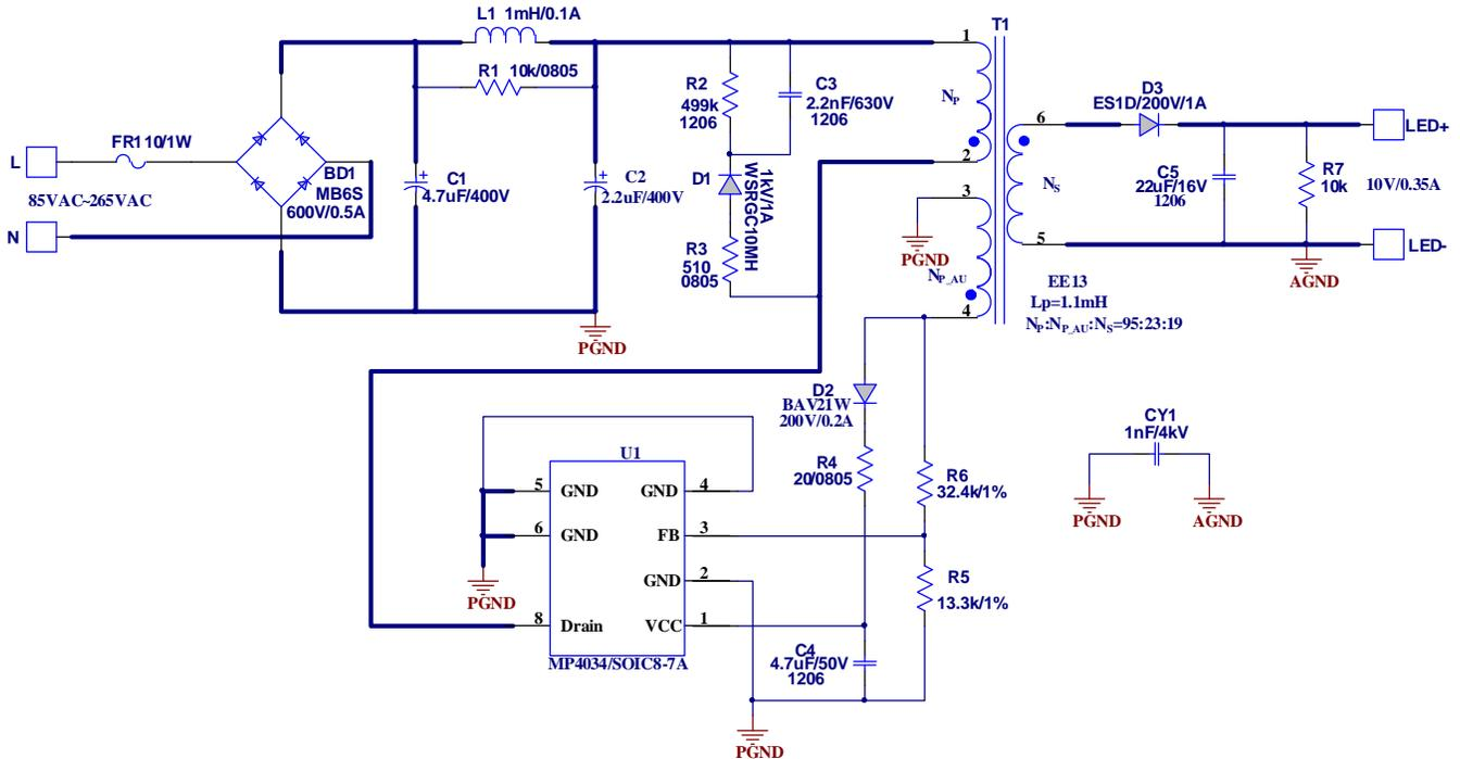
Figure 15: Typical Application Example
