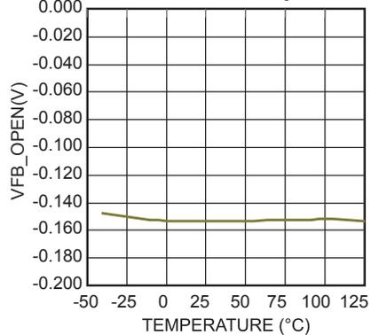
**Second-Level OVP Threshold vs. Junction Temperature**
