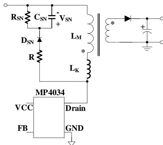
Figure 11: RCD Snubber
