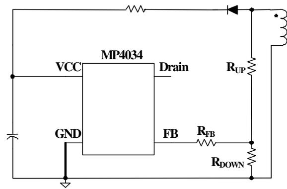
Figure 12: FB Pin in Series with ON Resistor
