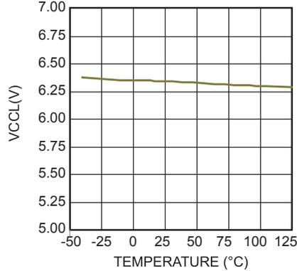
**First-Level OVP Threshold vs. Junction Temperature**
