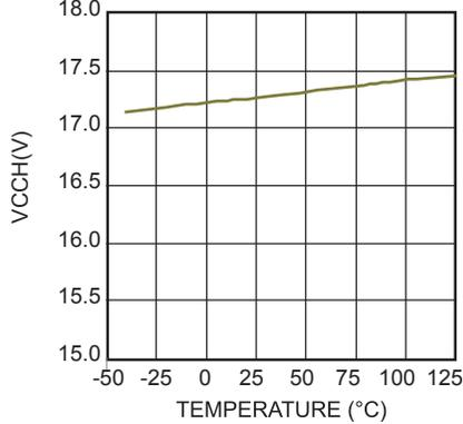
**V<sub>CC</sub> OFF Threshold vs. Junction Temperature**
