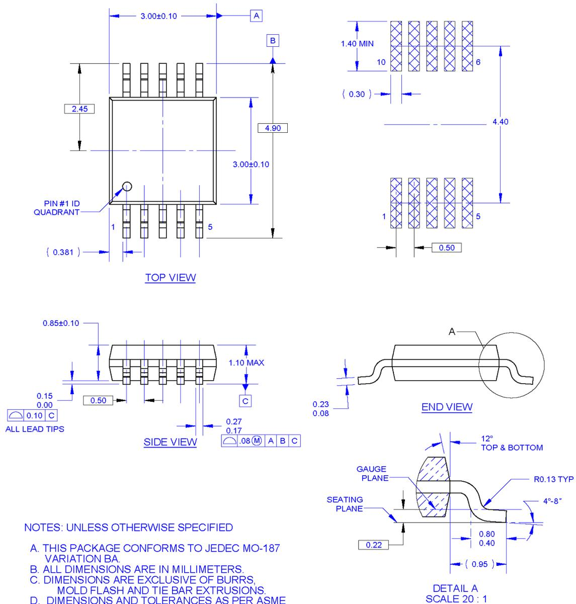
Figure 17. 10-Lead, Molded Small Outline Package (MSOP)
