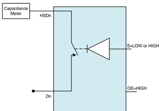
**Figure 14. Channel Off Capacitance**
