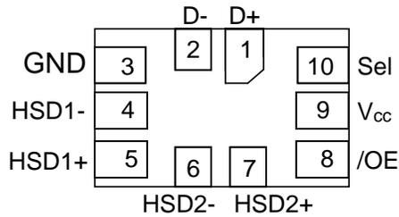
Figure 2. 10-Lead UMLP (Top-Through View)
