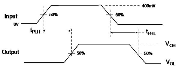
Figure 8. Propagation Delay ( $t_{rTF} = 500$  ps)
