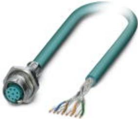
Assembled Ethernet cable, shielded, 4-pair, AWG 26 stranded (7-wire), RAL 5021 (sea blue), M12 flush-type socket, rear wall/screw mounting with M16 thread on free cable end, line, length 0.5 m
