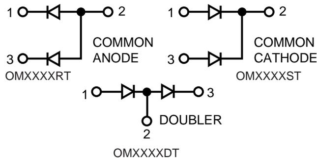
Common cathode is standard. Contact the factory for performance characteristics for common anode and doubler.
