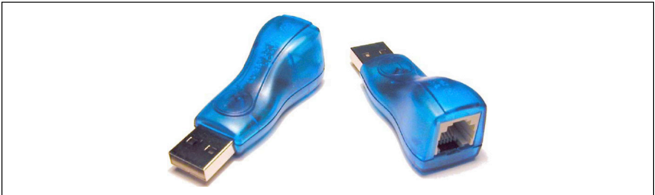
Figure 2. DS9490R# USB-to-1-Wire/iButton Adapter
